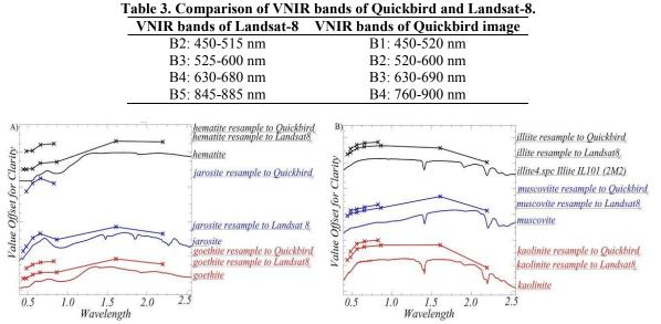
Figure 5. Spectral plots of some minerals extracted from USGS spectral library and resample to band centers of Landsat-8 and Quickbird. A) Some iron oxide/hydroxide/sulfate minerals B) some clay minerals.
