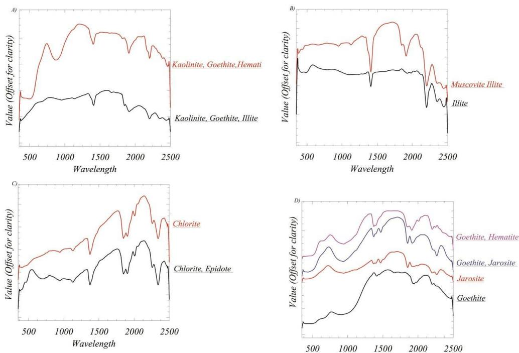
Figure 3. Different types of alteration minerals identified by spectroscopic studies A) argillic B) phyllic C) propylitic D) gossan.
