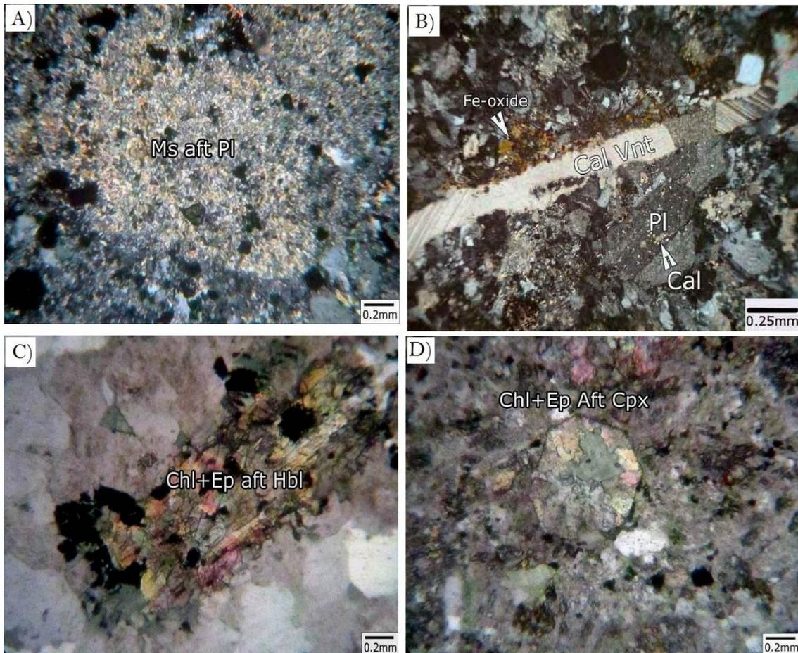
**Figure 4. Microscopic thin sections of some samples observed in crossed polarized light A) Plagioclase phenocrysts are pervasively replaced by muscovites B) Veinlet of calcite with iron oxide C) Hornblane phenocrysts are replaced by chlorite and epidote D) Clinopyroxen phenocrysts are replaced by chlorite and epidote.**
