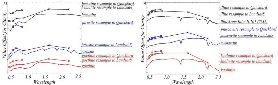
**Figure 5. Spectral plots of some minerals extracted from USGS spectral library and resample to band centers of Landsat-8 and Quickbird. A) Some iron oxide/hydroxide/sulfate minerals B) some clay minerals.**
