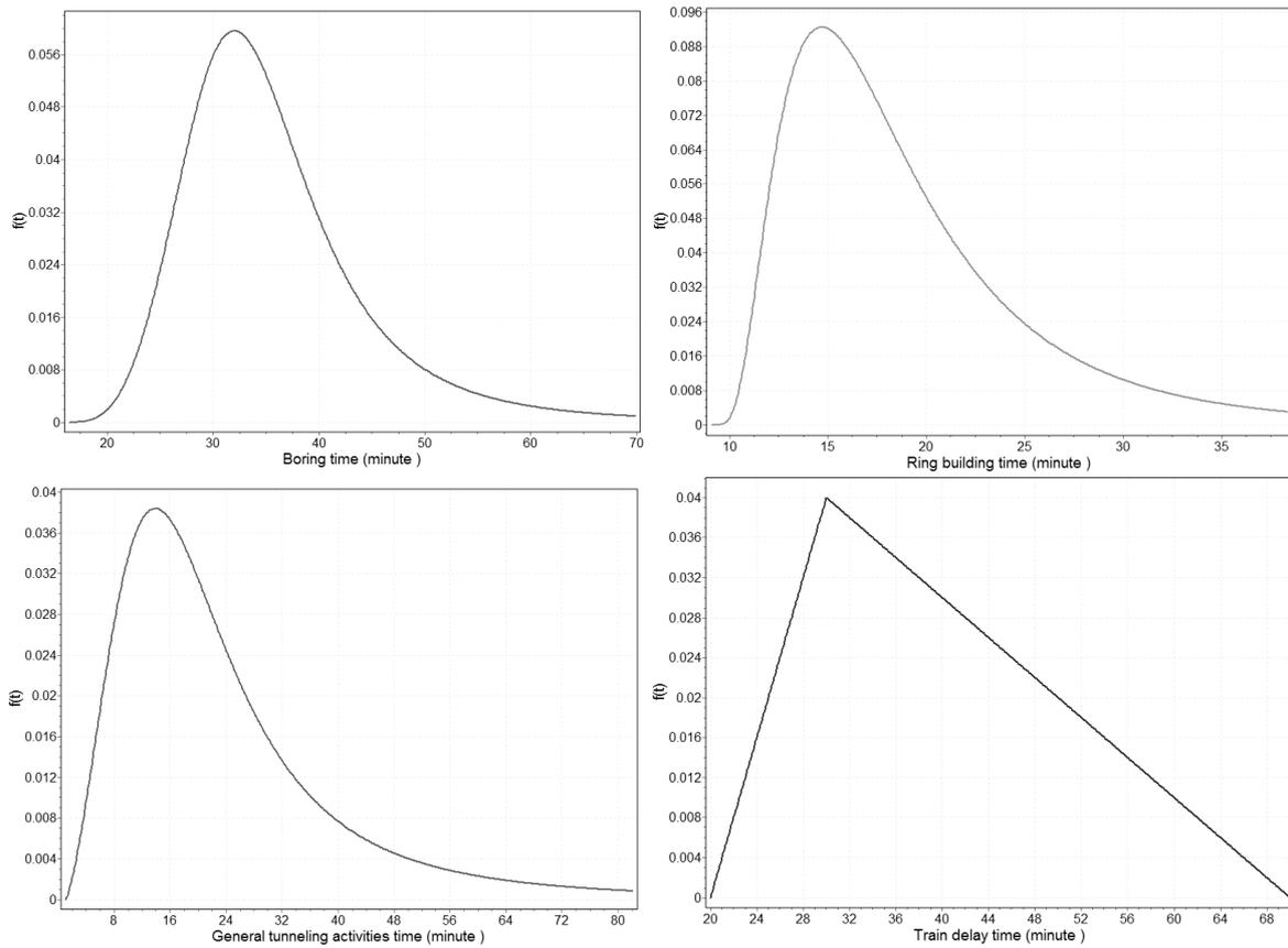
Figure 4. Probability density function plot of TBM production cycle activities.
