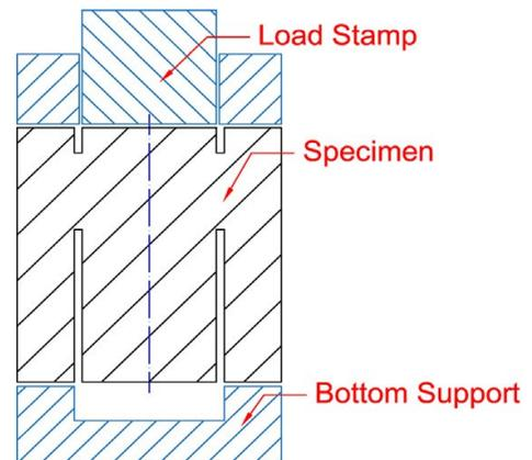
Figure 7. General schematic representation of loading [32].
