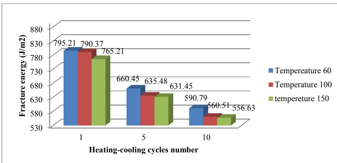
Figure 13. Changes in fracture energy with temperature and number of heating-cooling cycles.
