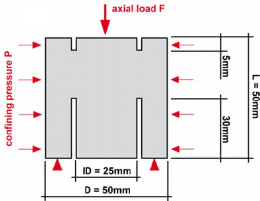
Figure 4. General form of specimen under stress [29].
