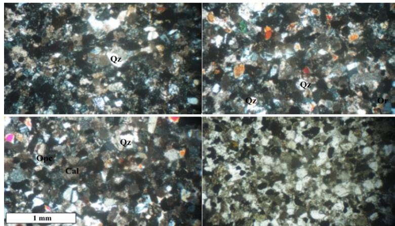
Figure 3. Microscopic images of sandstone specimen.
