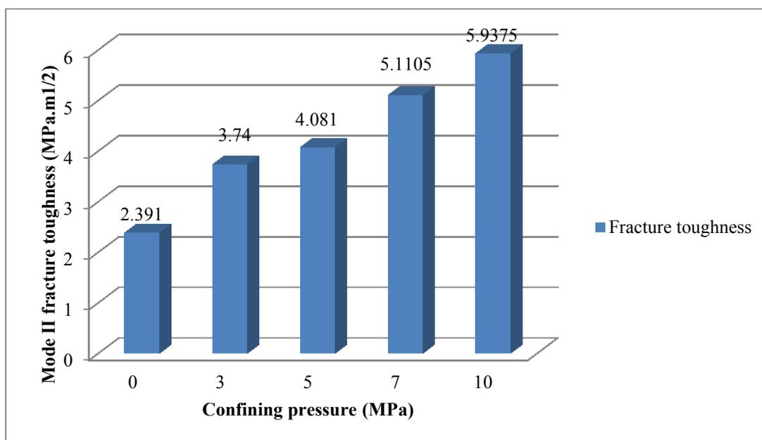
Figure 10. Changes in fracture toughness in the presence of confining pressure.
