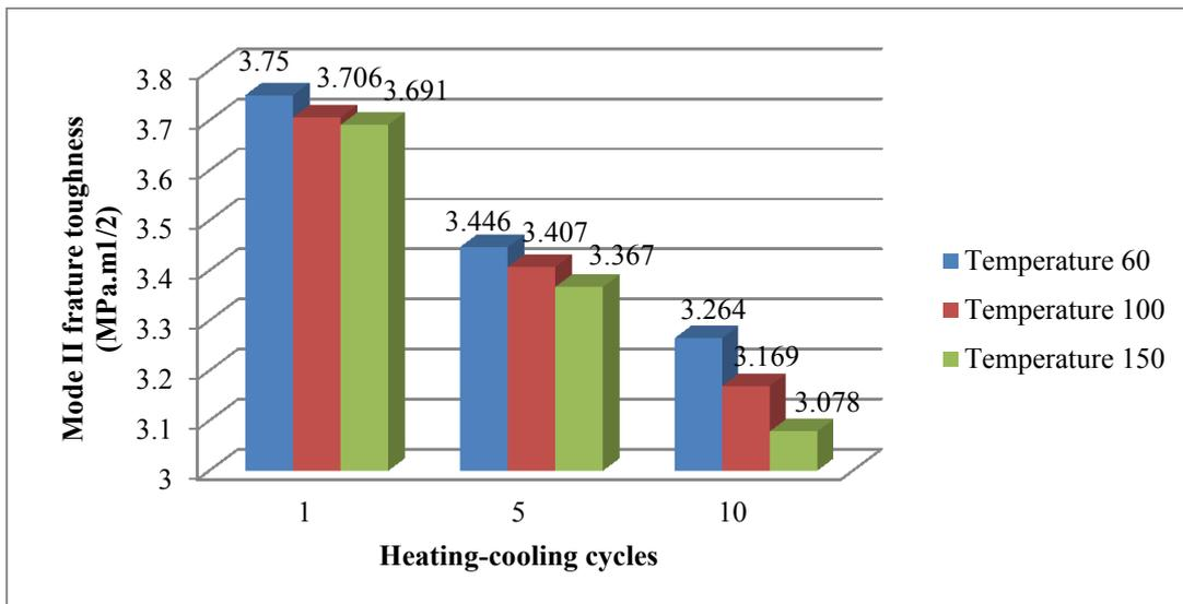
Figure 12. Changes in fracture toughness with temperature and number of heating-cooling cycles.
