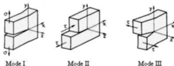
Figure 1. Fracture modes [11].
