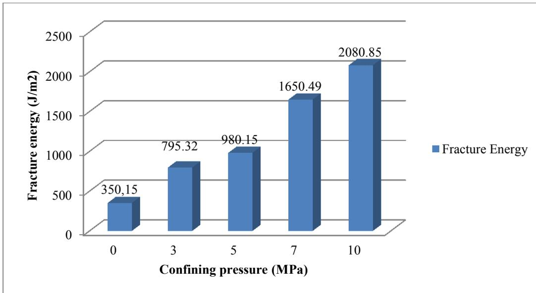
Figure 11. Changes in fracture energy in the presence of confining pressure.
