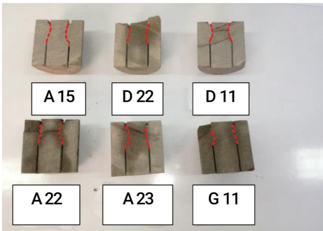
Figure 14. A profile of fracture propagation of specimens (cracks generated after test are marked in red).
