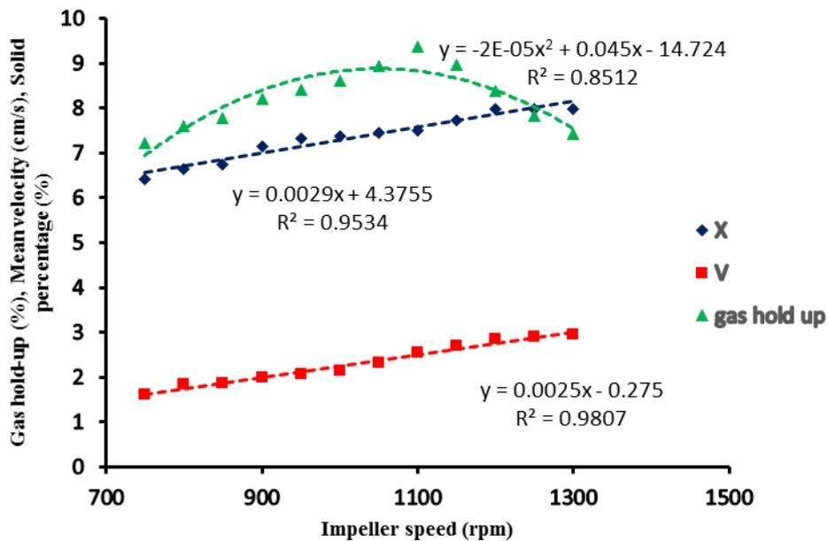
Figure 11. Relationship between impeller speed and properties of quiescent zone.
