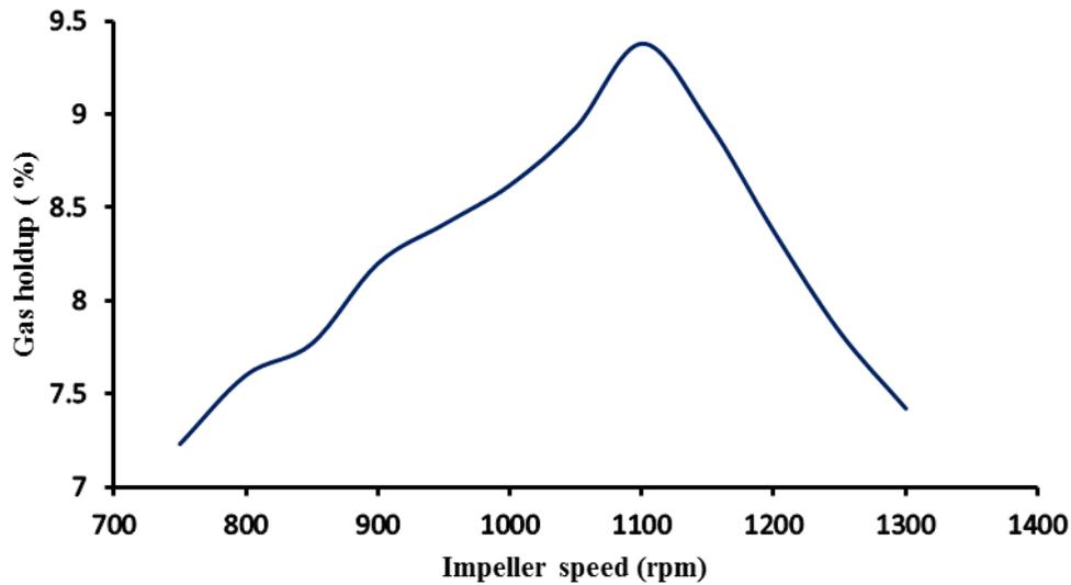
Figure 6. Effect of impeller speed on gas hold-up in quiescent zone.
