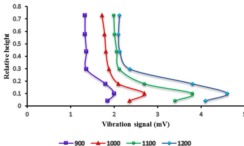
Figure 3. Relationship between impeller speed and height of quiescent zone.
