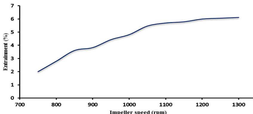
Figure 8. Relationship between entrainment and impeller speed.
