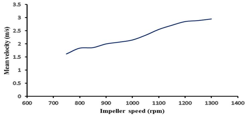
Figure 4. Effect of impeller speed on turbulence of quiescent zone.
