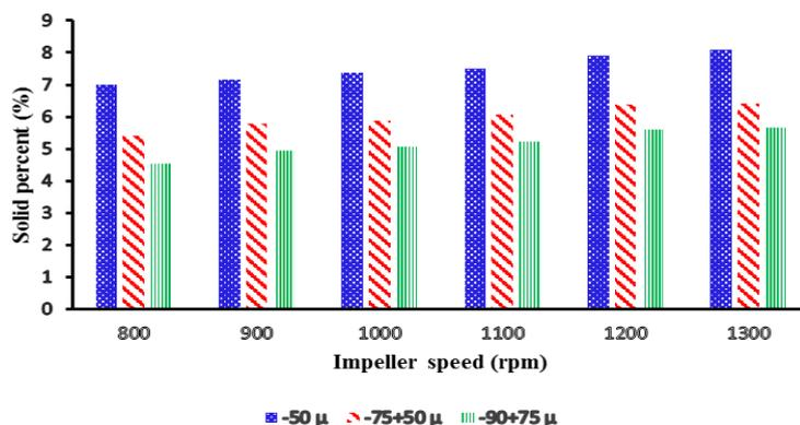
Figure 5. Effect of impeller speed on amount of transferred materials to quiescent zone in case of the three size fractions.
