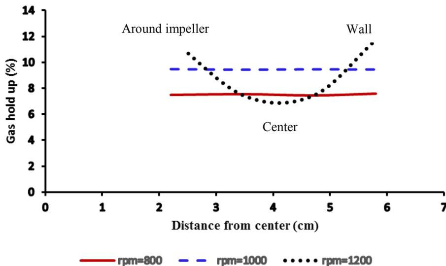
Figure 7. Local gas hold-up values measured at different distances around impeller shaft within quiescent zone for different impeller speeds.
