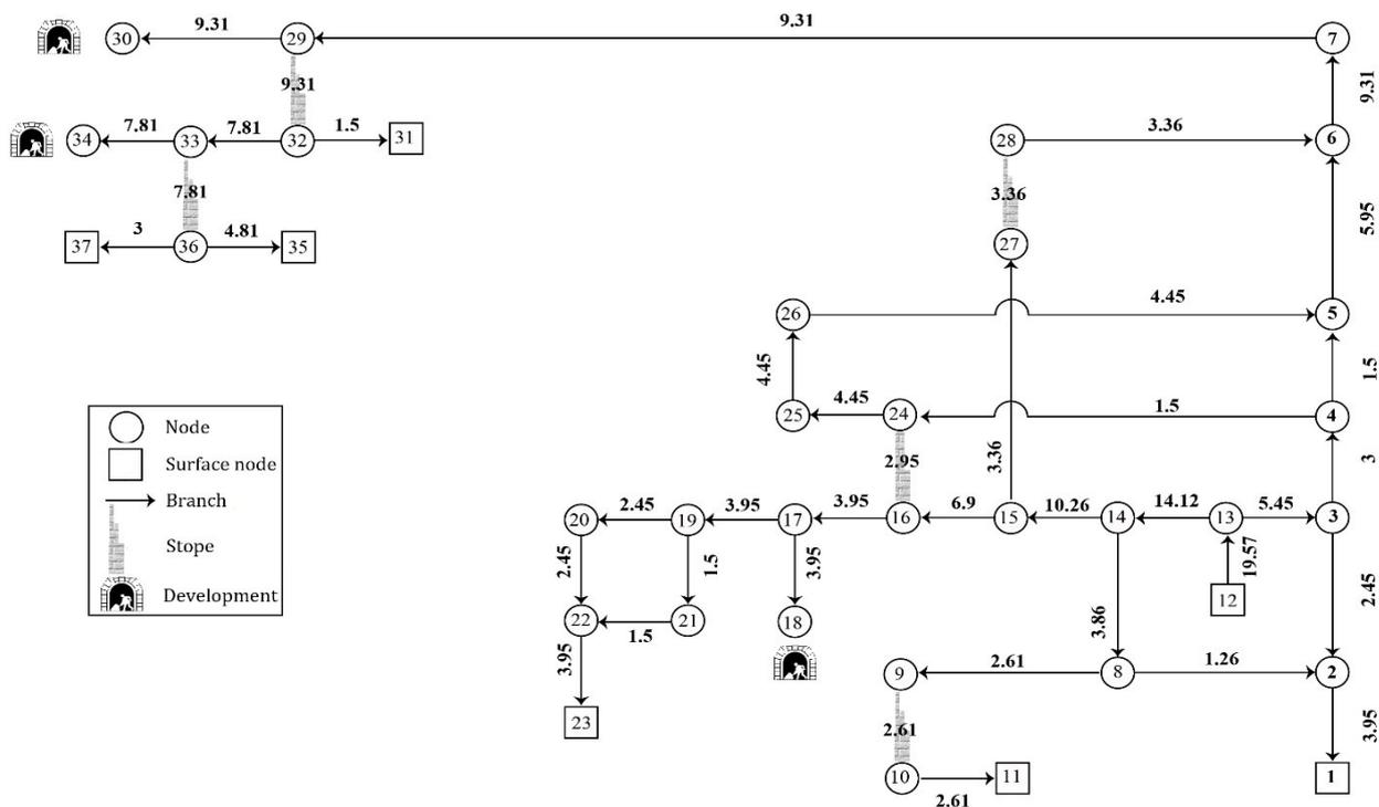
**Figure 2. Airflow distribution for entire mine ventilation network (m<sup>3</sup>/s).**
