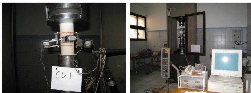
Figure 3. UCS test using MTS testing machine equipped with lateral chained LVTD displacement sensors.
