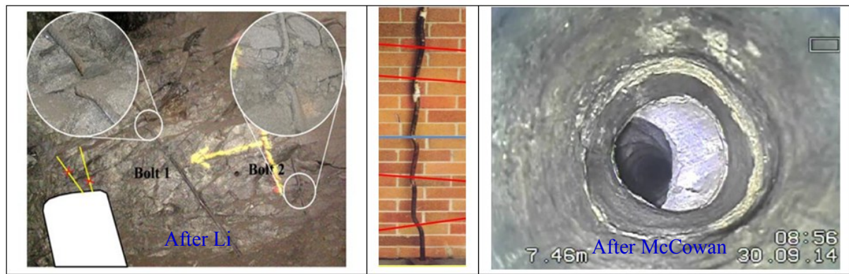
Figure 1. Sheared tendons recovered from field and a hole view of sheared rock [7, 8].
