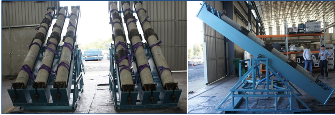
Figure 4. Tilting the pre-tensioned cables in concrete cylinders during the grouting stage.
