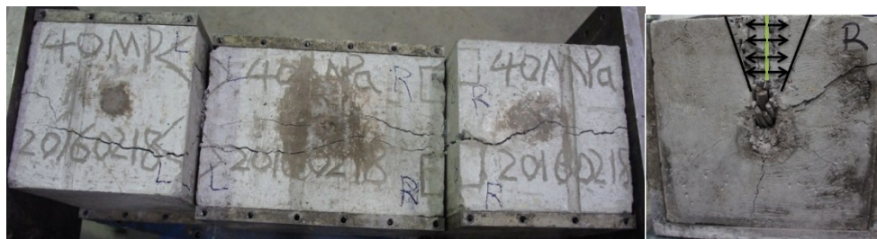
Figure 12. Double shear post-test concrete blocks crack.
