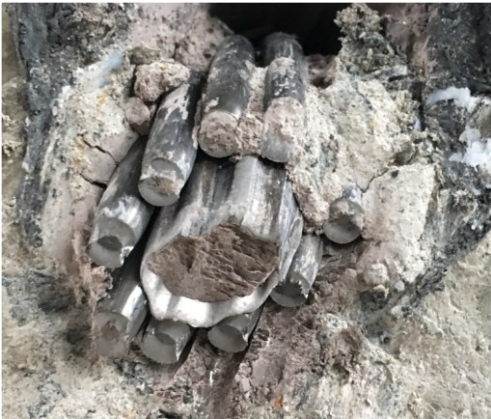
Figure 15. Cross-sectional view of de-bonded Plain MW10. Note the extent of wire failure in tension with failed wires surface being mostly in cone and cup.
