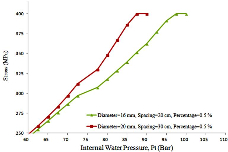
Figure 6. Comparison among stresses at different levels of high water pressure for the cases of the same steel ratio.
