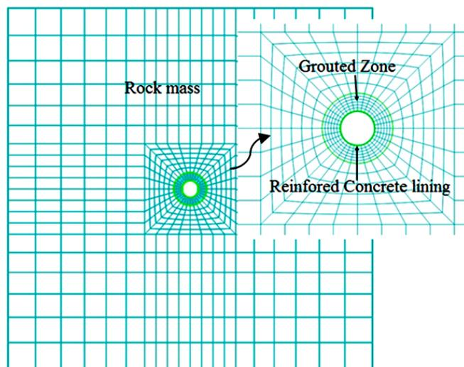
Figure 1. Finite element model.
