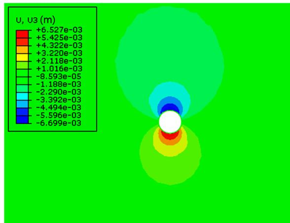
Figure 3. Displacement in the roof of tunnel before the applied internal water pressure.
