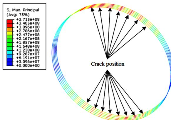
Figure 5. Increasing the stress on the steel bars under internal water pressure in the locations of lining.
