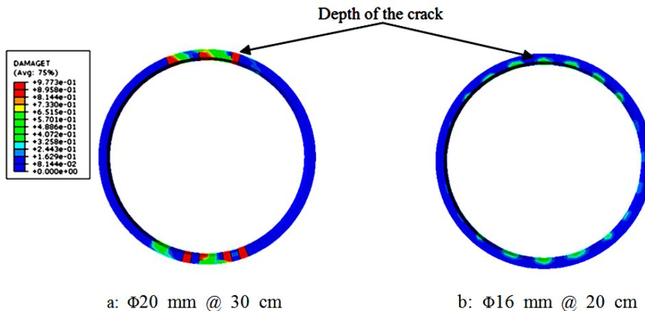
Figure 8. Comparison between the properties (depths and number) of cracks.
