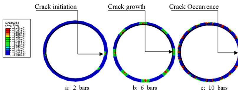
Figure 4. Development of cracks in the concrete lining under internal water pressure.
