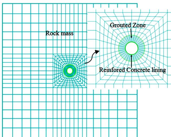
Figure 1. Finite element model.
