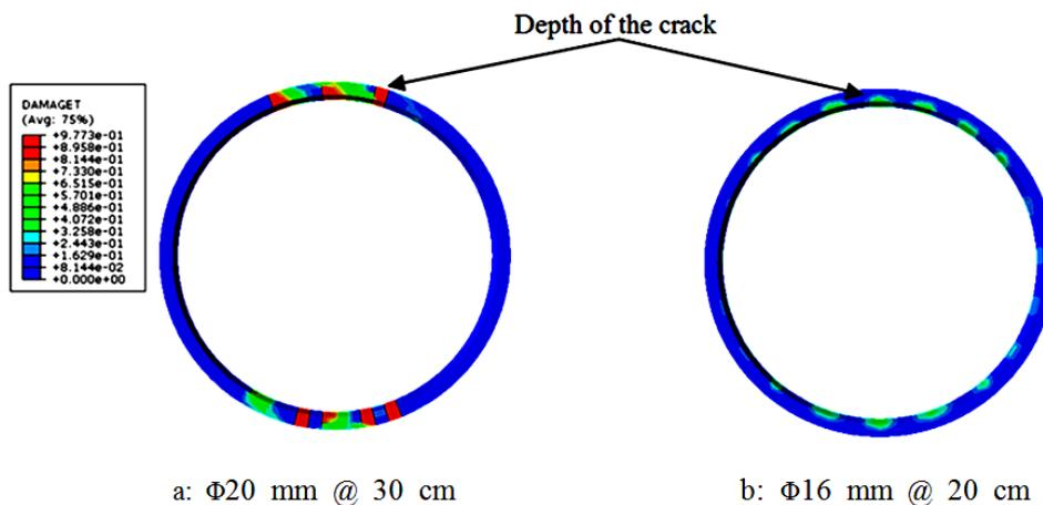
Figure 8. Comparison between the properties (depths and number) of cracks.
