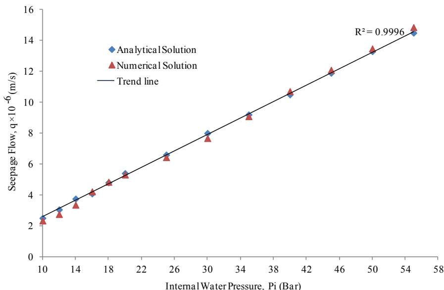
Figure 2. A comparison between the results of the analytical and numerical methods in the seepage flow calculation.
