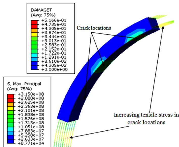
Figure 9. Increasing tensile stress at the location of cracking in concrete lining.
