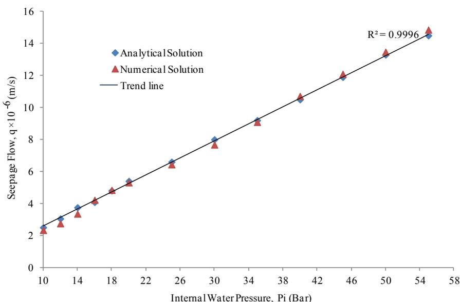
Figure 2. A comparison between the results of the analytical and numerical methods in the seepage flow calculation.
