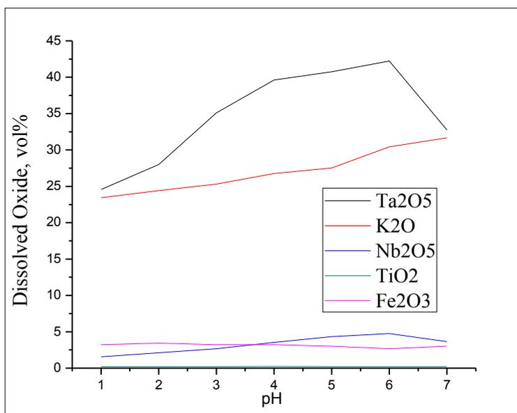
**Figure 3. Compositional analysis of leached liquor using ICP-OES.**
