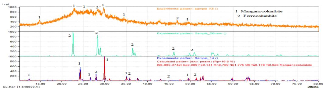
Figure 4. Compositional XRD spectra for Ta<sub>2</sub>O<sub>5</sub> (sample A5) and Nb<sub>2</sub>O<sub>5</sub> (sample D6).
