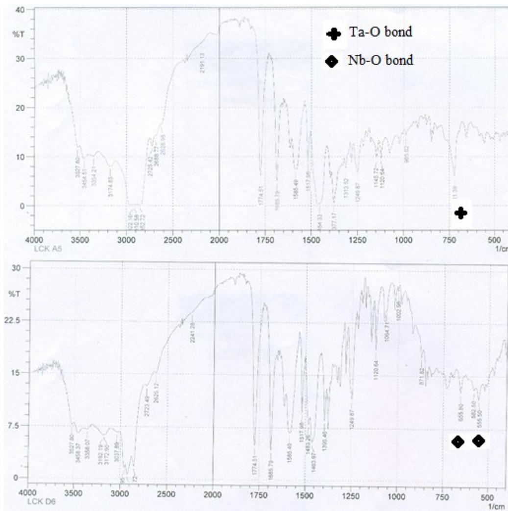
Figure 5. FI-IR stretching frequencies of Ta<sub>2</sub>O<sub>5</sub> (sample A5) and Nb<sub>2</sub>O<sub>5</sub> (sample D6).
