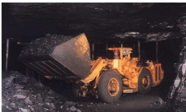
Figure 2. A typical LHD vehicle performing a loading operation.
