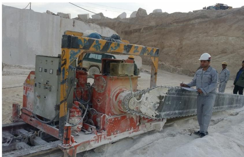
Figure 2. The chain saw machine used in this work.
