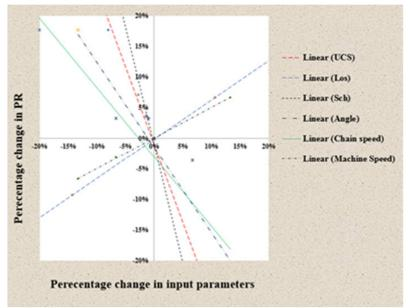
Figure 15. Sensitivity analysis based upon measured production rate.
