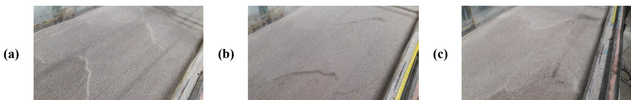
Figure 3. Pit infilling at the end of the tests at \frac{L}{y} = 12 , a) \frac{S}{B} = 50\% , b) \frac{S}{B} = 35\% c) \frac{S}{B} = 20\% .
