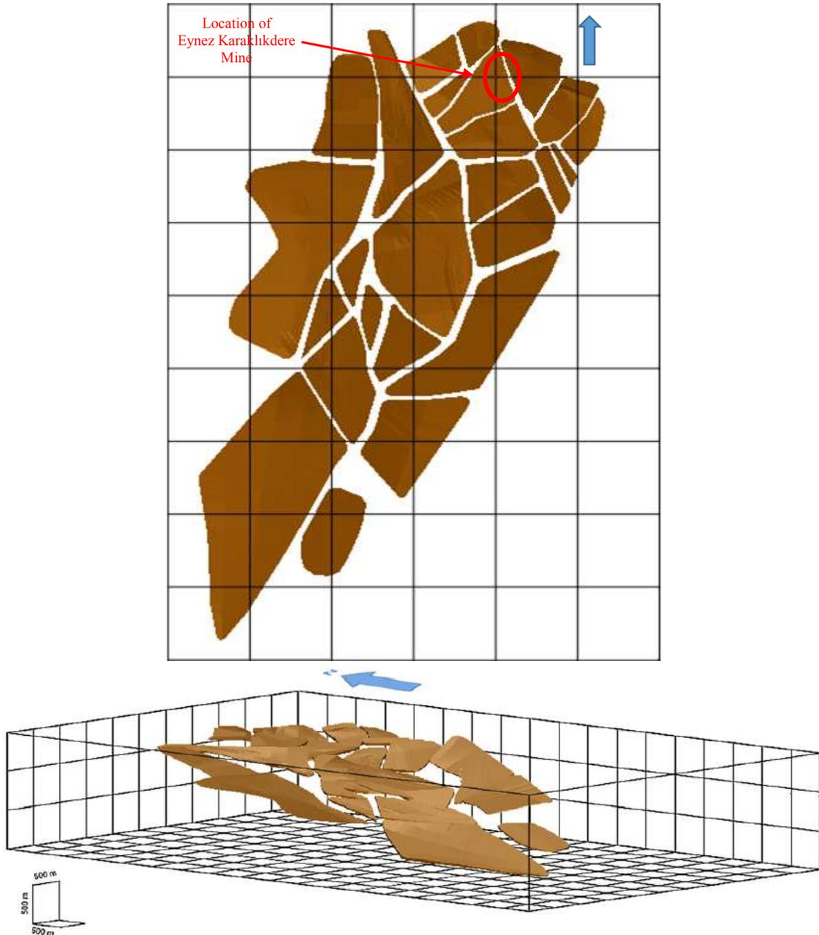
Figure 3. Plan and isometric views of the coal blocks separated by faults in Eynez field [4, 5].
