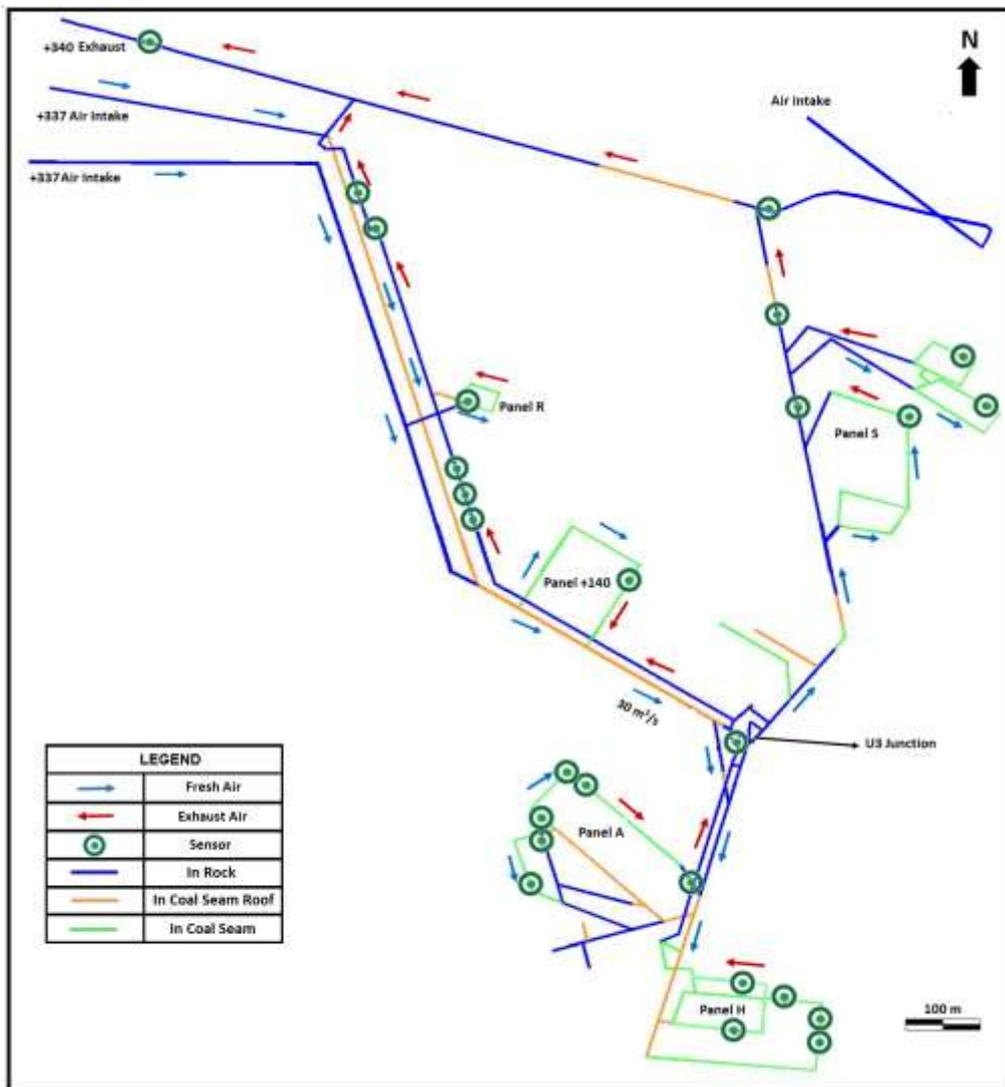
Figure 5. Eynez Karanlıkdere underground mine plan showing locations of operating panels, sensor locations, and ventilation (modified from [8]).
