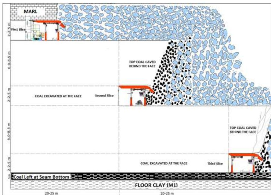
Figure 4. Cross-sectional view of LTCC production method applied at Eynez field (modified from [8]).
