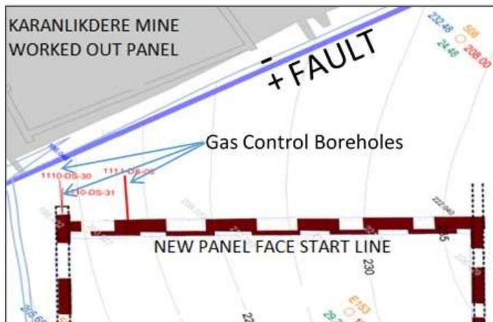
Figure 16. Locations of gas control boreholes opened towards old workings of Karanlıkdere mine.
