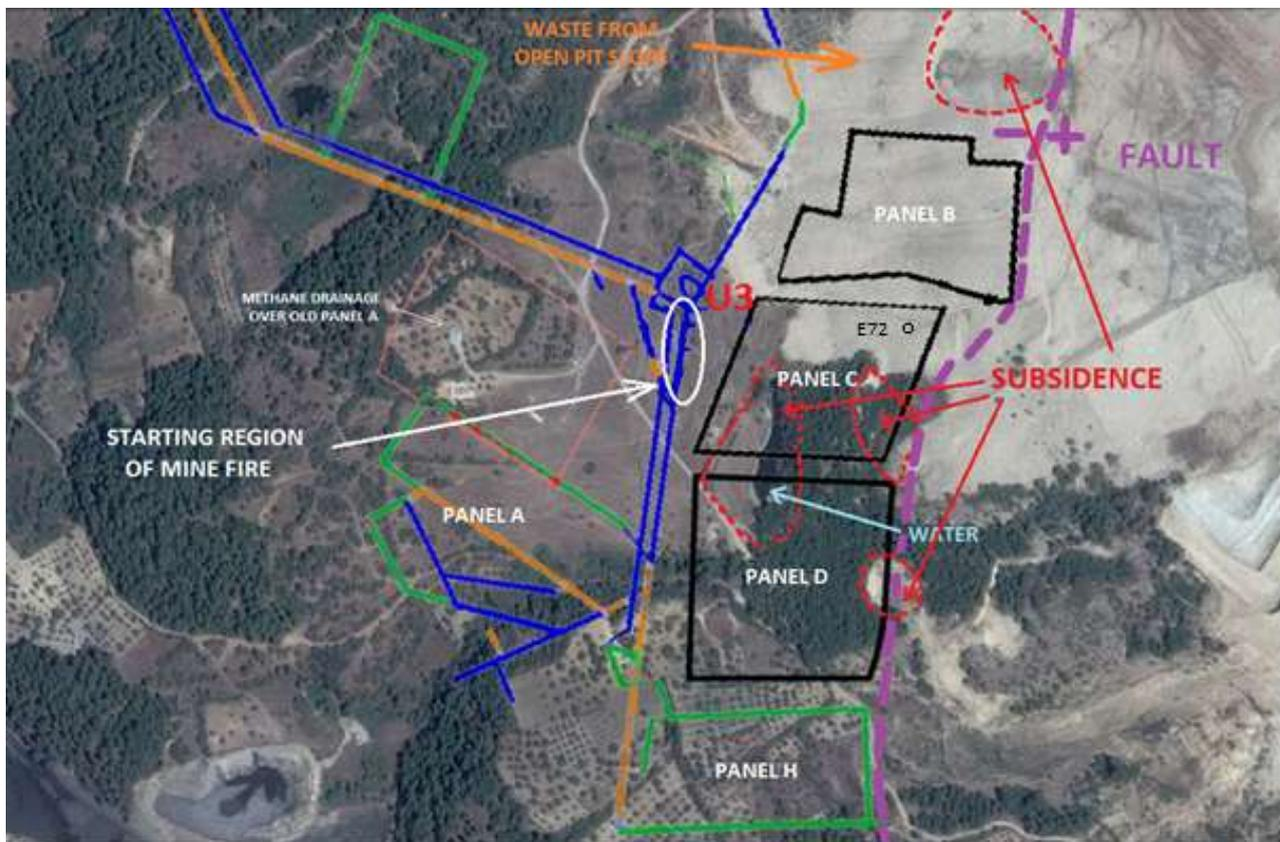
Figure 10. Details of mine plan on satellite image.
