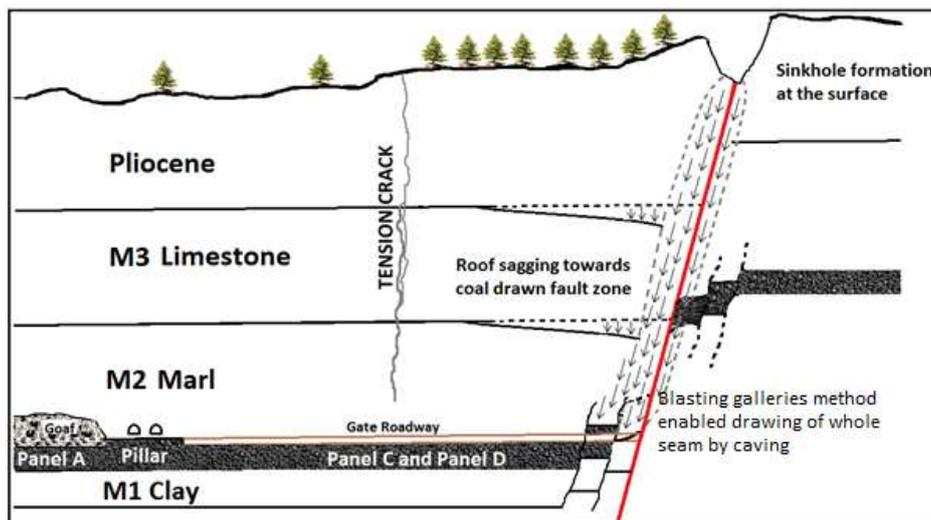
a) Formation of sinkhole due to full stamp caving of coal at fault contact and formation of tension crack in the middle due to diminishing of constraint on roof strata at fault side.
