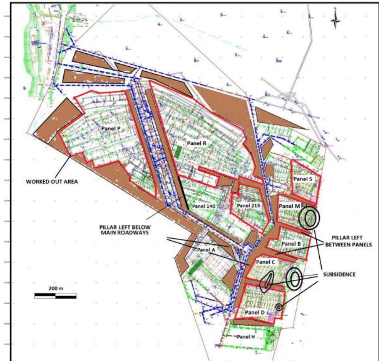
Figure 6. Mine plan showing old and active production areas, protective pillars, and locations of excessive subsidence observed at the surface (modified from [8]).
