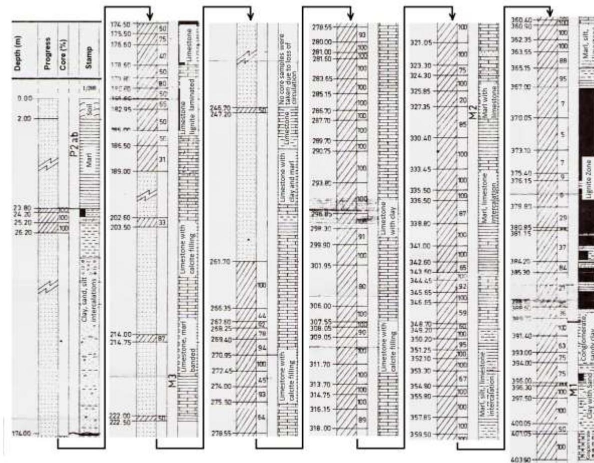
Figure 11. Log of the surface exploration borehole E72 opened on panel C.
