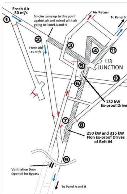
Figure 8. A close-up plan of mine fire start region (modified from [8]).
