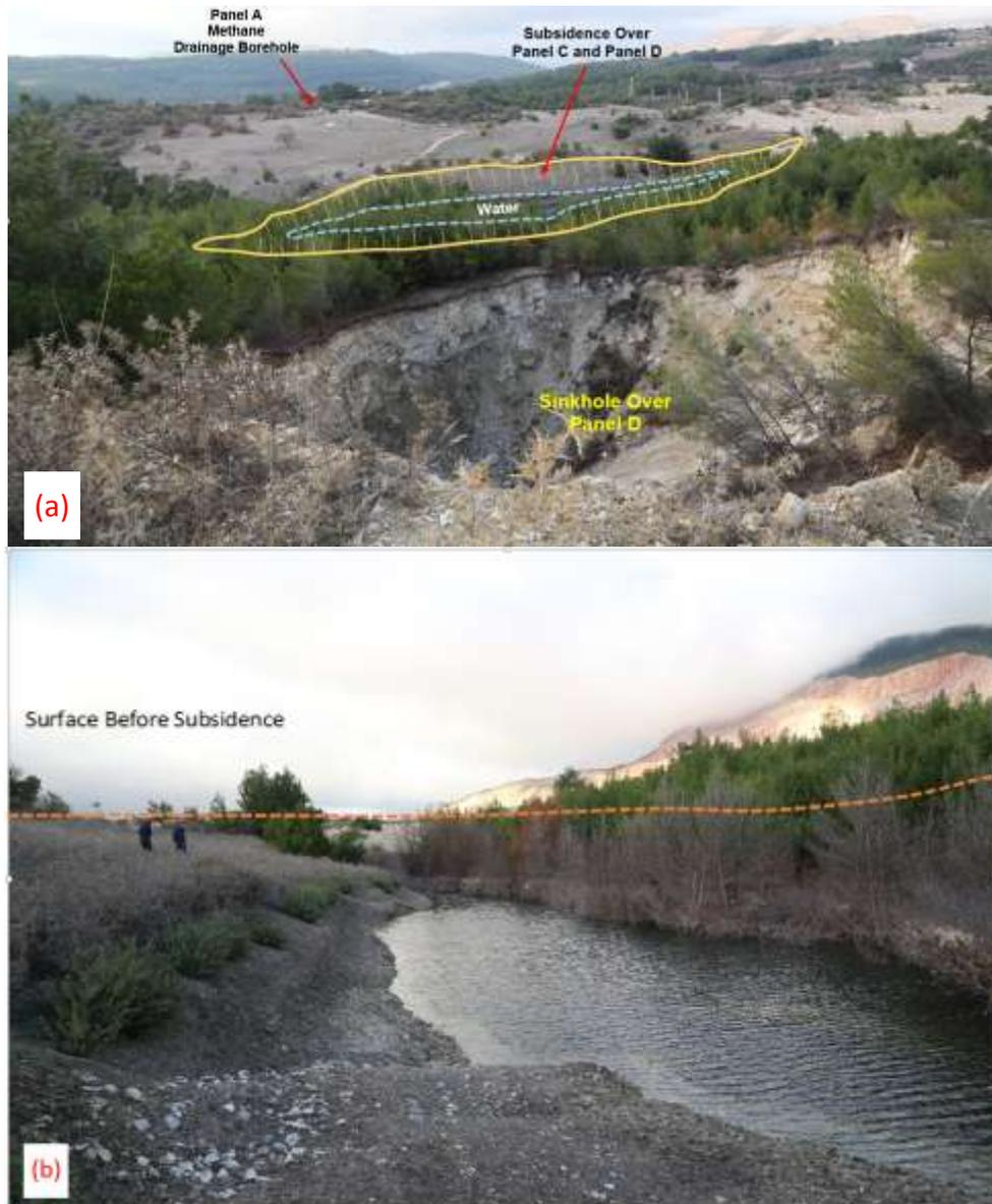
Figure 13. a) Sinkhole over panel D fault contact, and b) water filled subsidence wedge formation across panel D and panel C.
