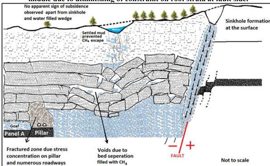
b) Caving of roof after production of three slices resulting in void formation filled with methane due to bed separation and unconsolidated goaf.
