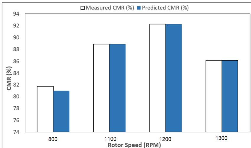
Figure 15. The predicted and experimental effects of rotor speed on CMR: conditioning time, 3 min; gasoline dosage, 300 g/ton; pH, 8; flotation retention time, 3 min; solid weight content, 15%; frother dosage, 25 g/ton; and feed ash, 43.9%.
