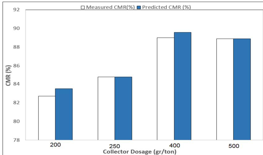
Figure 16. The predicted and experimental effects of gasoline (collector) dosage on CMR: conditioning time, 3min; rotor speed, 1200 RPM; pH, 8; flotation retention time, 3 min; solid weight content, 12%; frother dosage, 81 g/ton; and feed ash, 43.87%.
