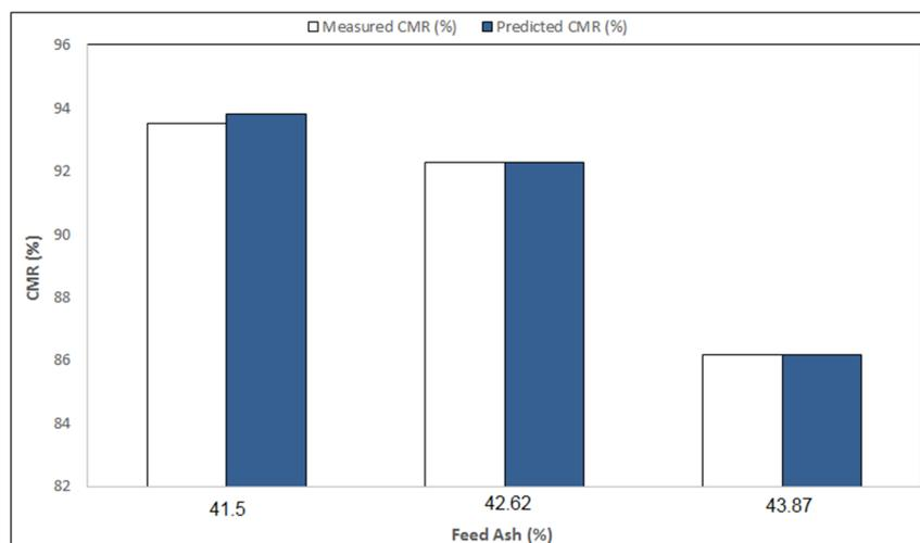
Figure 18. The predicted and experimental effects of feed ash on CMR: conditioning time, 3 min; rotor speed, 1200 RPM; pH, 8; flotation retention time, 3 min; collector dosage, 500 g/ton; frother dosage, 81g/ton; and solid weight content, 15%.
