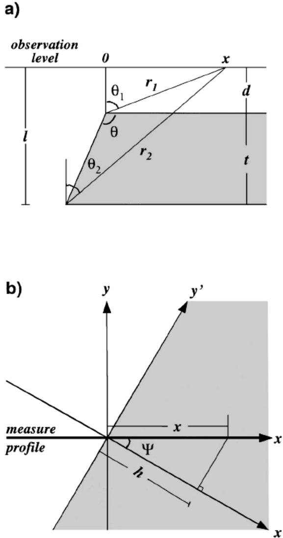
Figure 1. (a) Cross-sectional view of a step model. (b) Plane view of the step model whose strike is along the y-direction, but the survey is supposed to be conducted along the x-direction.
