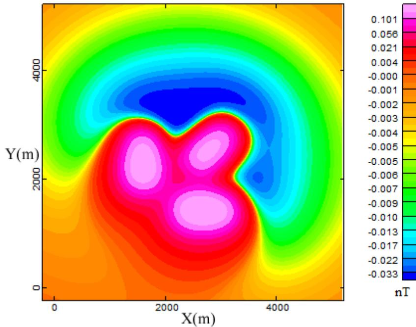
Figure 2. Magnetic response from three prismatic models with vertical sides in different depth and inclination.
