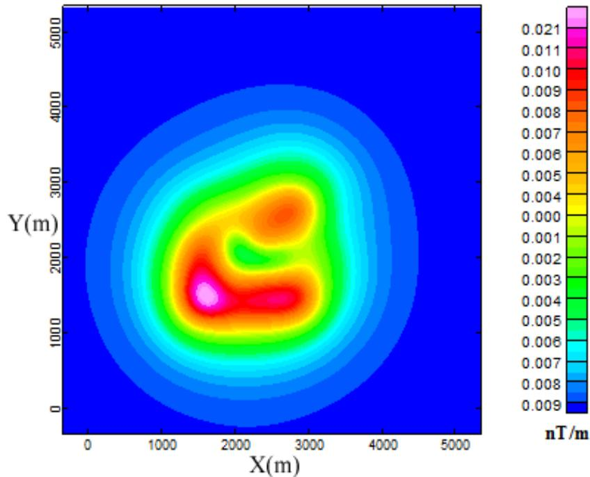
Figure 3. Boundaries detection of three models in Figure 2 using simple analytic signal.
