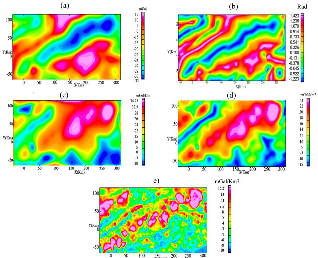
Figure 6. Application of the proposed filters on gravity data of southwest England: (a) Bouguer gravity map of the study area; (b) Theta map of the data in Figure 6a.; (c) Analytic Signal map of the gravity in Figure 6a.; (d) First – order vertical derivative of the analytic signal; (e) Second – order vertical derivative of the analytic signal.
