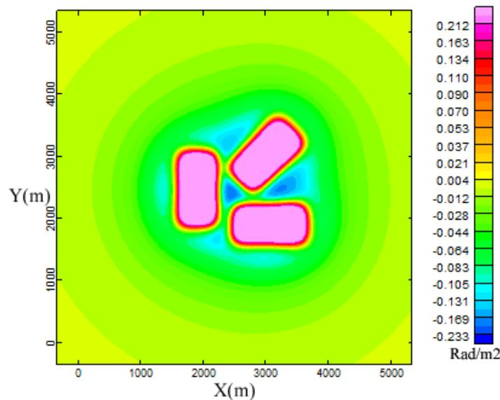
Figure 4. Boundaries detection of three models in Figure 2 using second- order vertical derivative of analytic signal.
