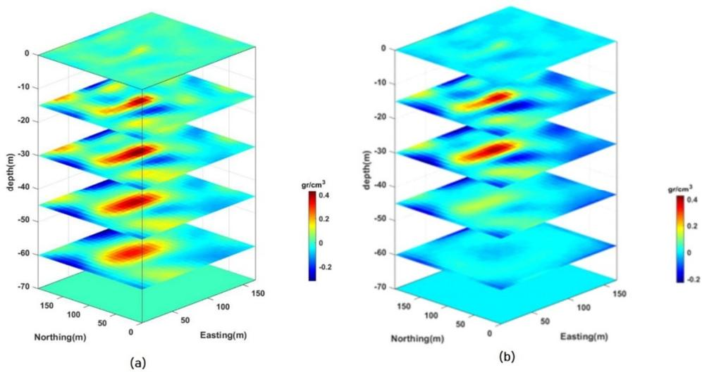
Figure 6. (a) Plan sections through the recovered density models obtained from the 3D smooth inversion of gravity anomaly using the GCV method at different depths. (b) The ACB method.
