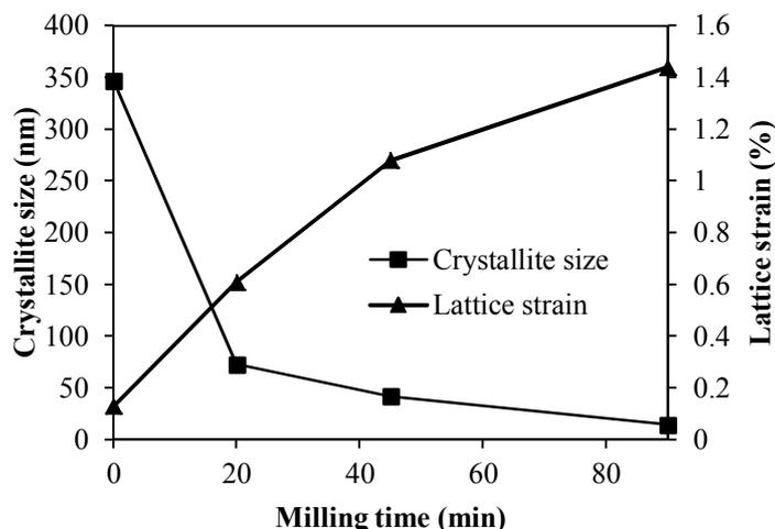
Figure 6. Crystal lattice strain increase and ilmenite crystal size decrease as functions of mechanical activation duration.
