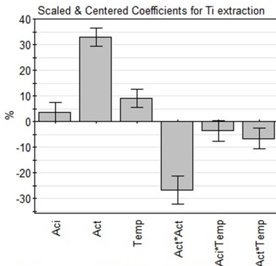
Figure 10. Plot of model coefficients for titanium extraction.
