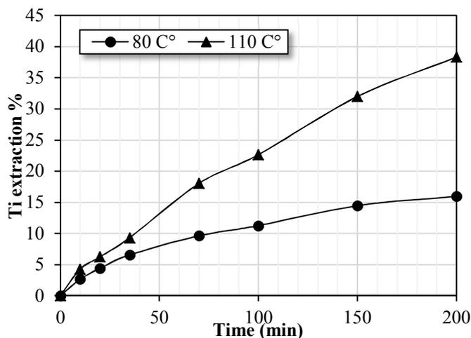
Figure 13. Effect of temperature on titanium extraction from non-activated ilmenite (acid = 55 wt.%).
