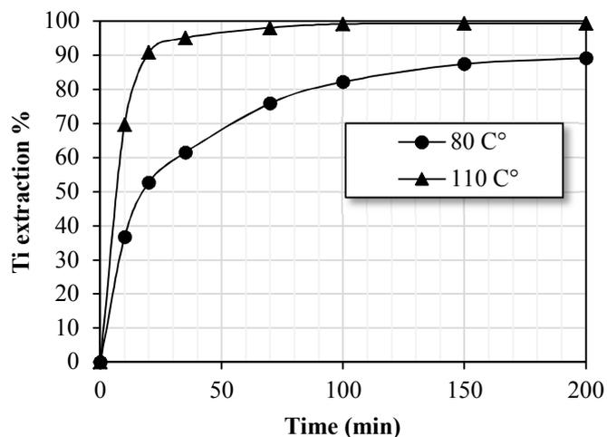
Figure 14. Effect of temperature on titanium extraction from activated ilmenite (acid = 55 wt.%).
