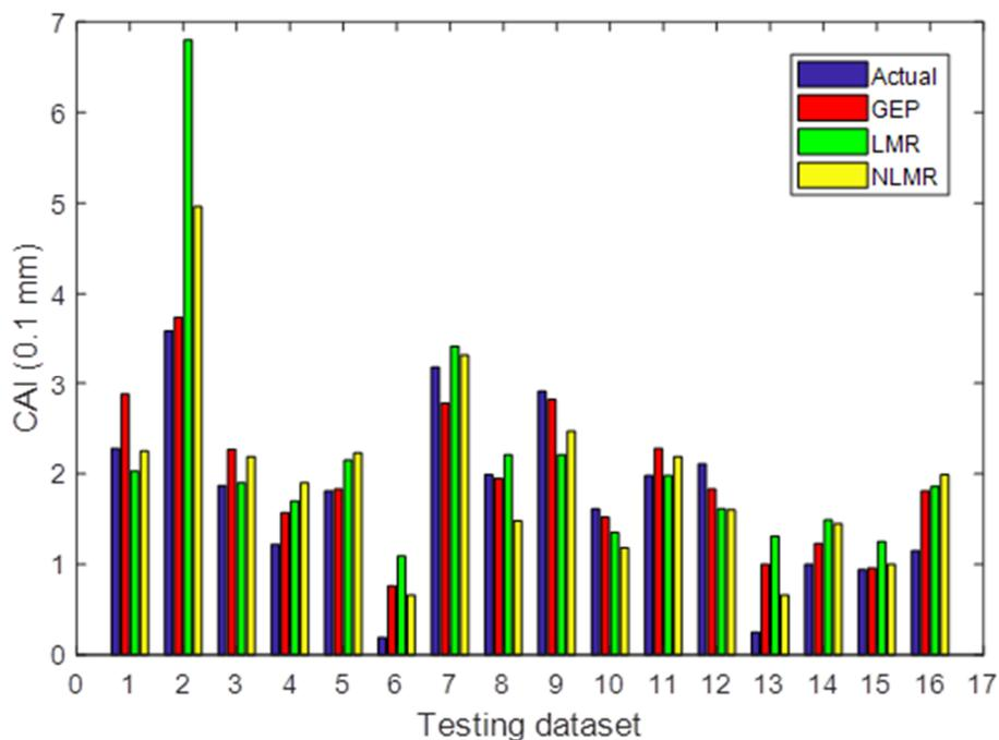
Figure 5. Comparison of the predicted CAI values using the GEP, LMR, and NLMR models and the actual CAI values.
