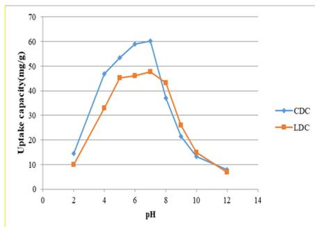
**Figure 7. Relation between adsorption capacity and different pH values.**
