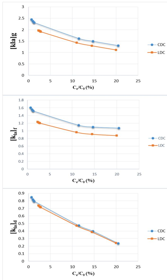
Figure 11. Variation in mass transfer factors: (a)  $[k_{1a}]_g$ , (b)  $[k_{1a}]_f$ , (c)  $[k_{1a}]_d$  for chloride ion adsorption onto CDC and LDC ( $C_0 = 250$  mg/L,  $T = 25$  °C, amount of adsorbent = 1 g).
