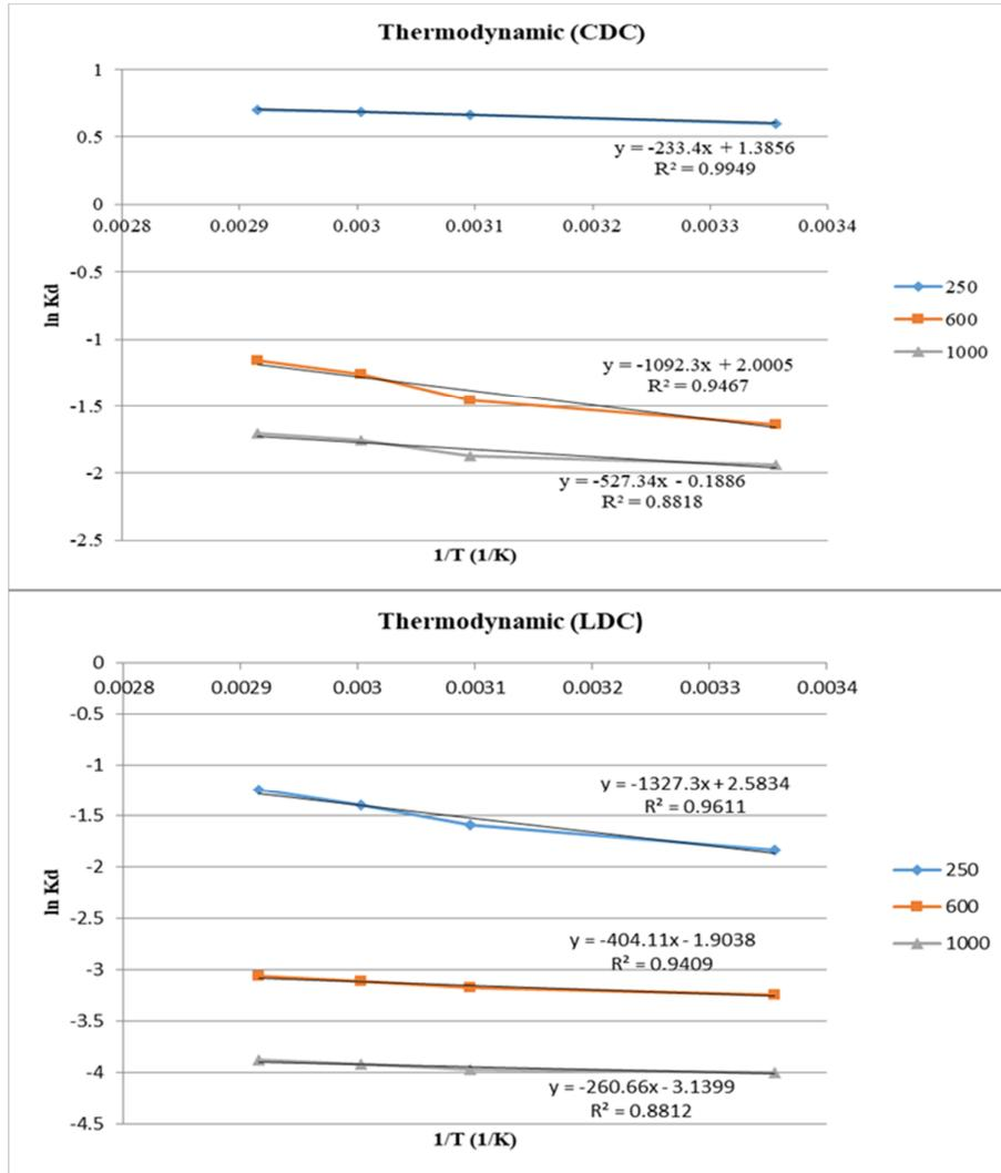
Figure 12. Plot of  $\ln K_d$  versus  $1/\text{temperature}$  to determine enthalpy and entropy of the adsorption reaction for CDC and LDC (initial chloride concentration: 1000, 600, 250 mg/L, speed stirrer: 500 rpm, temperature: 298 K, 323 K, 333 K, 343 K).
