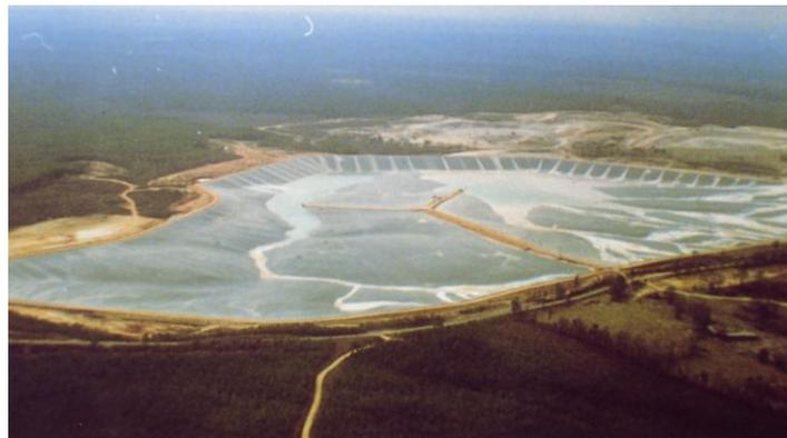
**Figure 4. A view of a typical tailings pond**
