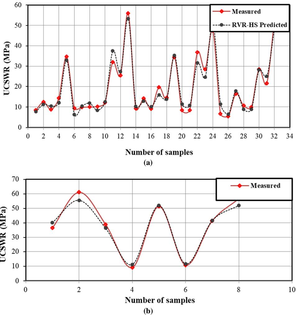
Figure 3. Correlation between the measured and estimated UCSWR using the RVR-HS model for a) training datasets b) testing datasets.
