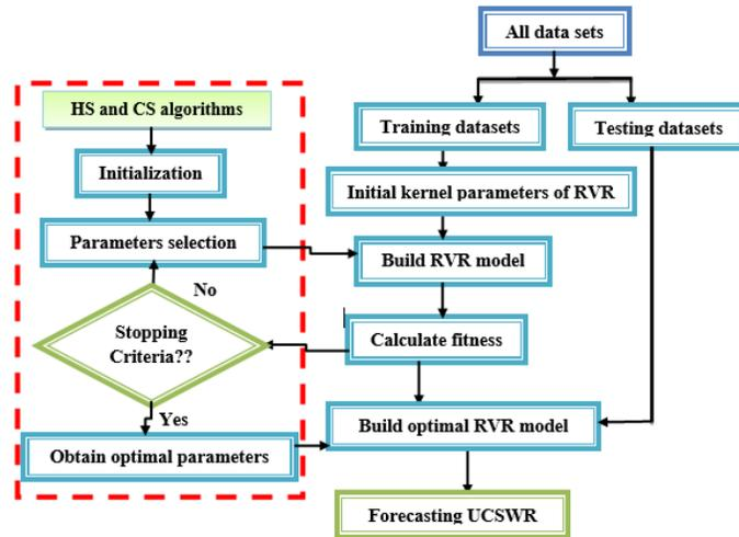
Figure 2. A flowchart of the RVR-CS and RVR-HS models for forecasting UCSWR.
