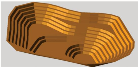
**Figure 6. A 3D view of the second push-back in the Chadormalu mine [34].**
