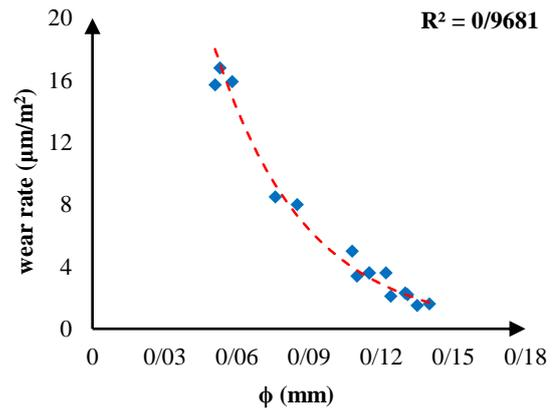
Figure 3. Exponential relation between measured wear rate and Grain size.
