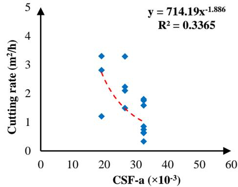
Figure 13. Correlation between  $CSF\_a$  (Table 5) and cutting rate.
