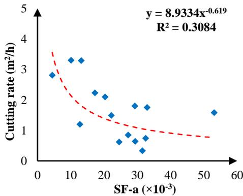
Figure 12. Correlation between  $SF\_a$  (Equation 1) and cutting rate.
