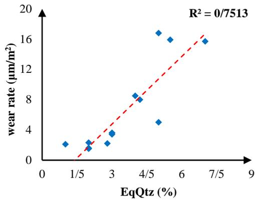
Figure 2. Linear relation between measured wear rate and EqQtz.
