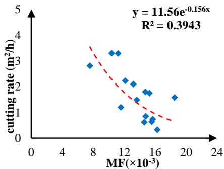
Figure 14. Correlation between  $MF$  (Equation 10) and cutting rate.
