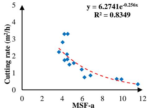
Figure 15. Correlation between  $MSF\_a$  (Equation 9) and cutting rate (present study).
