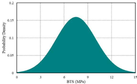
Figure 4. Normal distribution function used for Brazilian tensile strength.
