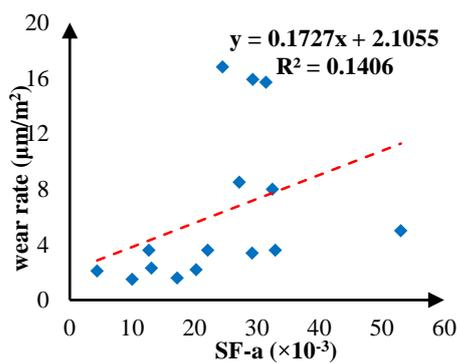
Figure 8. Correlation between  $SF\_a$  (Equation 1) and wear rate.
