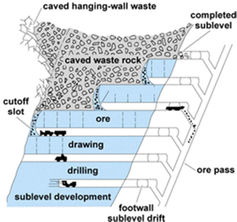
Figure 1. Sub-level caving mining cycle [13].
