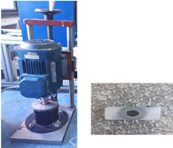
Figure 6. LCPC test machine (left), impeller after the LCPC test on andesite (right).
