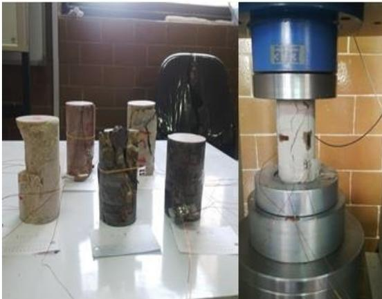
**Figure 4. Rock specimens fractured after the uniaxial compressive test.**
