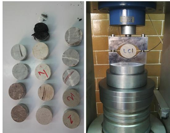
**Figure 5. Curved loading jaws of the Brazilian test (right) and rock specimens fractured after the Brazilian test (left).**
