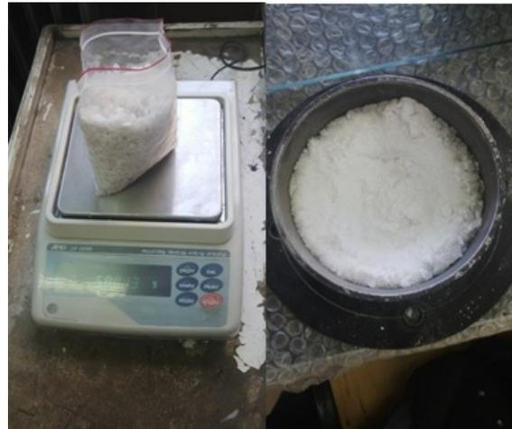
Figure 7. The salt rock sample before and after the LCPC test.
