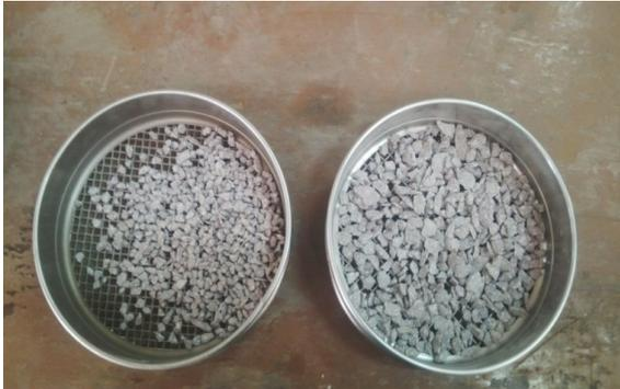
**Figure 3. Gyratory crusher output after separation. The left-hand side sample: the product passed through a 0.25" sieve remaining on a 5 mesh sieve, and the right-hand side sample: the product remaining on a 0.25" sieve.**
