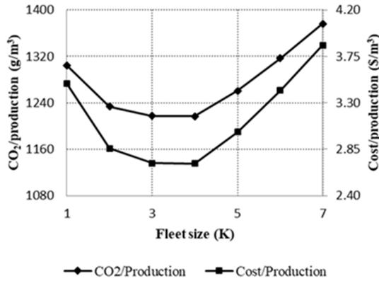
Figure 2. CO<sub>2</sub> EPP and CPP versus fleet size for doubling the service time of the case study.
