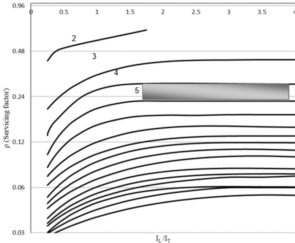
Figure 4. Optimum K based on the servicing factor and the ratio of the loader and truck's idling emissions.
