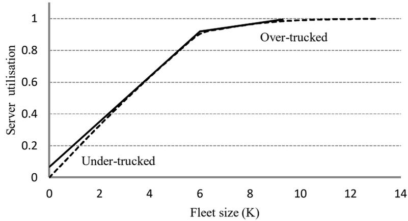
Figure 6. Example plot of server utilization (production) versus fleet size.
