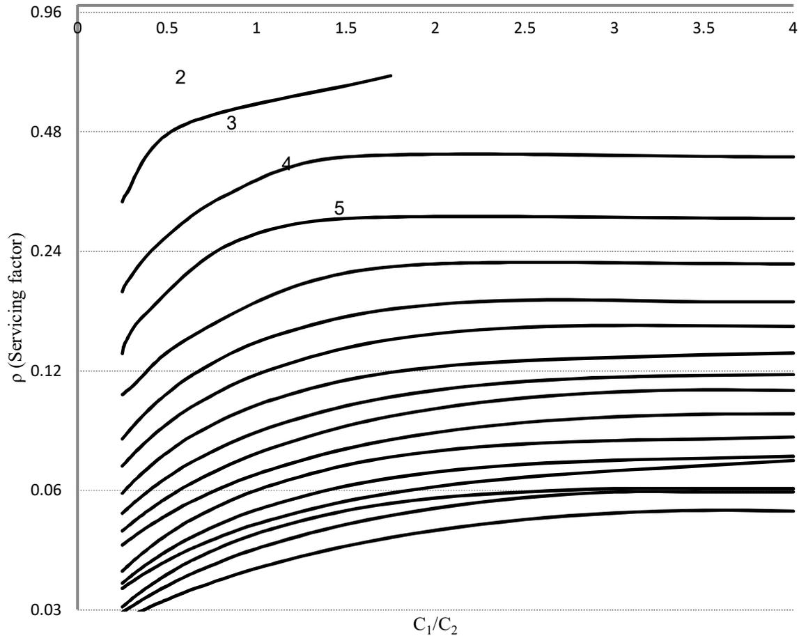
Figure 5. Optimum K based on the servicing factor and the ratio of the loader and truck’s costs.
