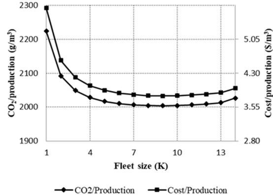
Figure 3. CO<sub>2</sub> EPP and CPP versus fleet for doubling the back-cycle time of the case study.
