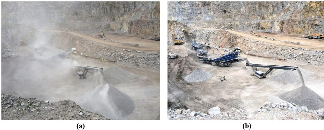
Figure 2. Effect of water spray on dust emission a) Before water spray and b) After water spray
