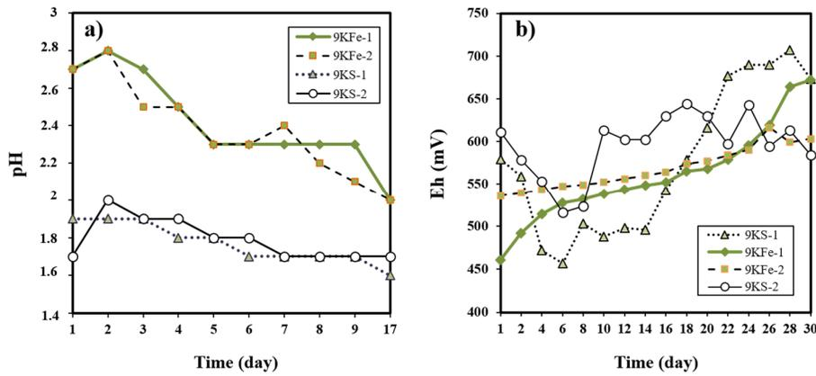
Figure8. a) Changes in pH over the time (days) for two identical 9KFe media and two identical 9KS media; b) Eh variations for bacteria growth in each 9KFe and 9KS medium.
