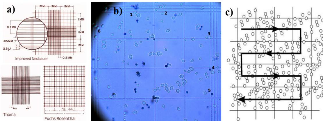
Figure5. a) Networking or hemocytometer of the Thoma counting chamber; b) The hemocytometer under the lens of the microscope; c) Route of the counting bacteria.
