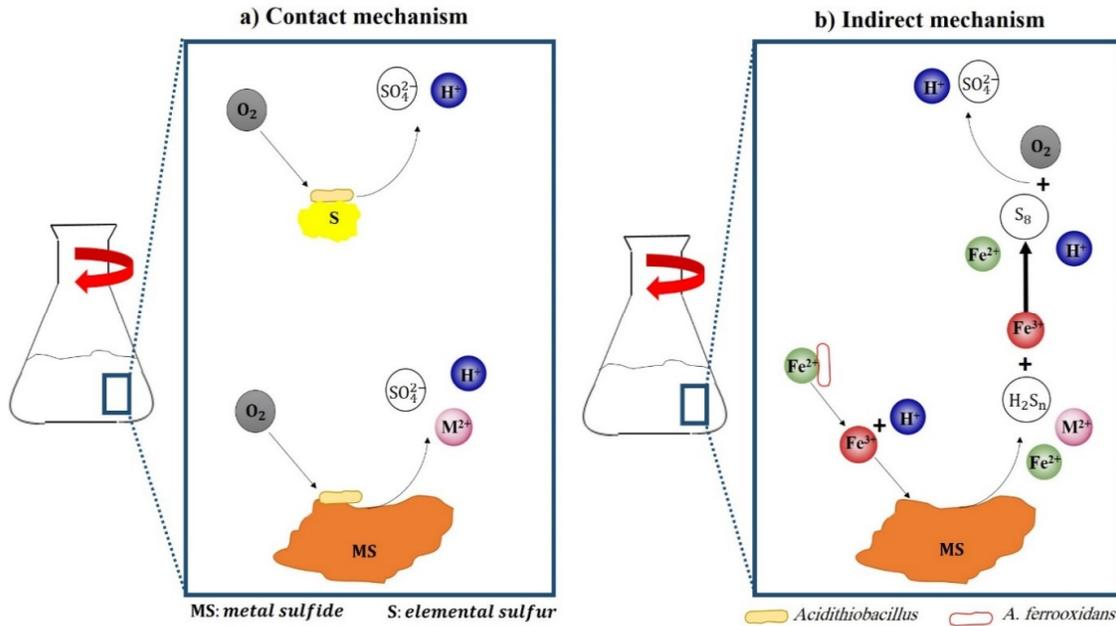
Figure 15. A schematic diagram for the mechanisms involved in acid production by the acidophilic bacteria a) contact mechanism; b) indirect mechanism.
