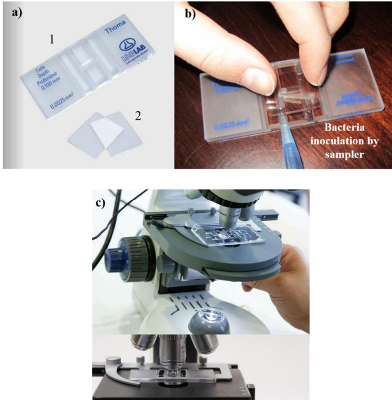
Figure4. a) Thoma counting chamber (1) and glass slide (2); b) Bacterial inoculation between the counting chamber and the glass slide for bacteria counting; c) Biological microscope (magnification of 40x is required for cell counting and 100x is useful to look at a larger grid in the hemocytometer).
