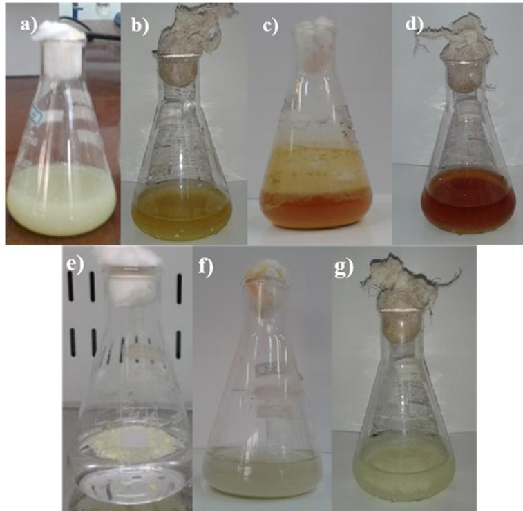
**Figure6.** Steps of color changes of 9K media during the growth of pure bacteria: a) Primary culture medium with a light color (green due to the presence of  $\text{Fe}^{2+}$  ions); b) Turbid solution compared to the primary culture medium (cream-brown color); c) Dark medium (reddish-brown); d) Final dark medium (dark red; rich in  $\text{Fe}^{3+}$  ions due to the bacterial activity); e) Colorless solution; f) Milky color; g) Clear cream-colored medium.
