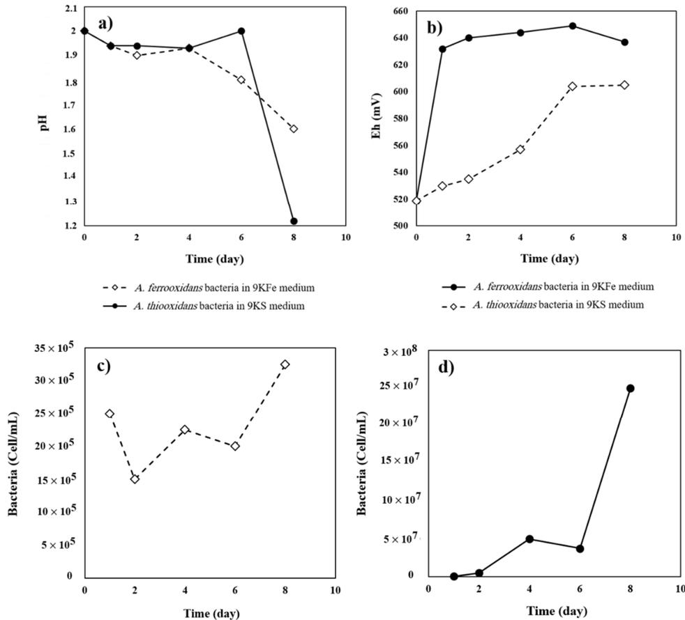
**Figure 14.** a) pH changes during the time; b) Eh changes over the time during the growth and proliferation of pure bacteria in the 9K medium; c) Changes in the number of *A.f* in the 9KFe medium during the time; d) variations in the *A.t* population over the time in the 9KS medium.
