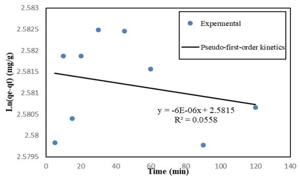
**Figure 19. Pseudo-first-order adsorption kinetics of CR18 onto nano-clay.**
