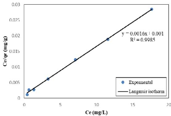
Figure 14. Plot of Langmuir isotherm for adsorption of CR18 onto nano-clay.
