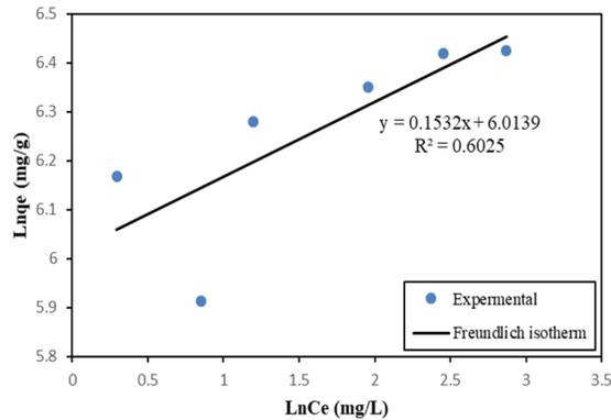
Figure 16. Plot of Freundlich isotherm for adsorption of CR18 onto nano-clay.
