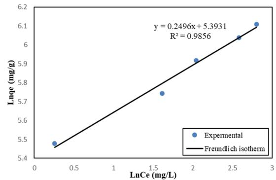
Figure 17. Plot of Freundlich isotherm for adsorption of CR18 onto Tonsil.
