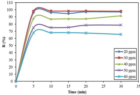
Figure 9. Effect of CR18 concentration on the adsorption efficiency of tonsil.
