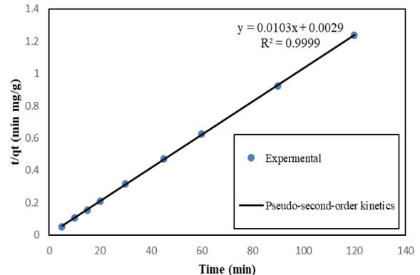
**Figure 21. Pseudo-second-order adsorption kinetics of CR18 onto nano-clay.**
