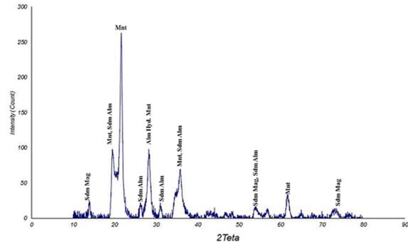
Figure 3. XRD graph for nano-clay.
