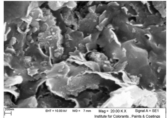
Figure 1d. SEM image of surface of the nano-clay adsorbent (Scale: 200 nm).
