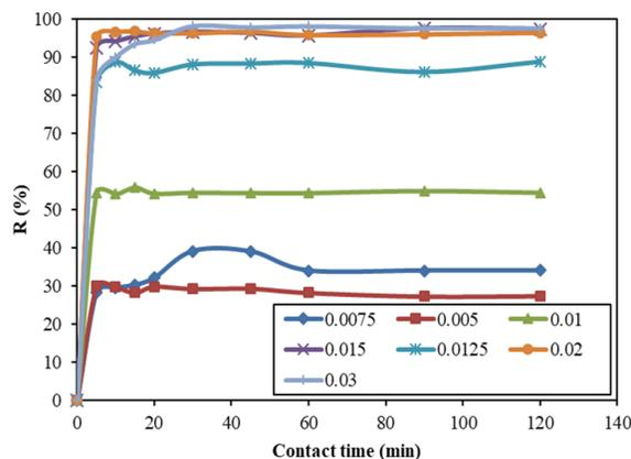
Figure 8. Effect of contact time on the adsorption efficiency of tonsil (0.005 and 0.0075), [dye] = 30 ppm.
