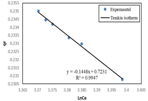
Figure 13. Plot of Temkin isotherm for adsorption of CR18 onto tonsil.
