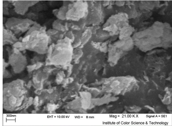
Figure 1b. SEM image of surface of the tonsil adsorbent (Scale: 300 nm).
