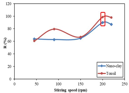
Figure 11. Effect of stirring speed on the adsorption efficiency.
