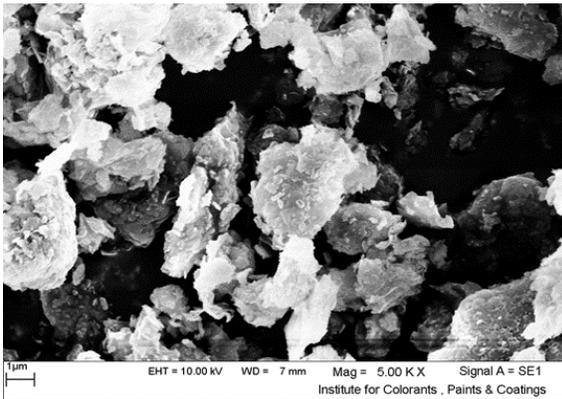
Figure 1c. SEM image of surface of the nano-clay adsorbent (Scale: 1 micron).
