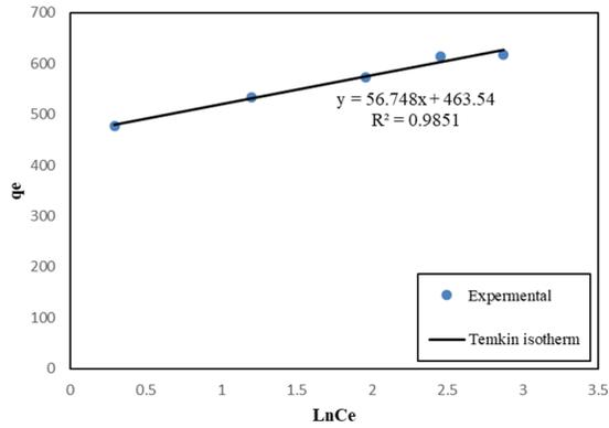
Figure 12. Plot of Temkin isotherm for adsorption of CR18 onto nano-clay.
