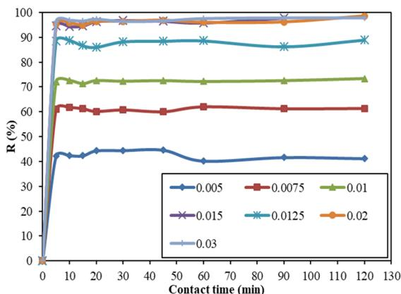
Figure 7. Effect of contact time on the adsorption efficiency of nano-clay, [dye] = 30 ppm.
