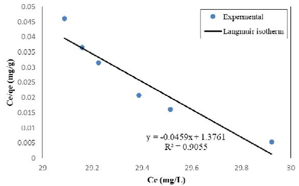
Figure 15. Plot of Langmuir isotherm for adsorption of CR18 onto tonsil.
