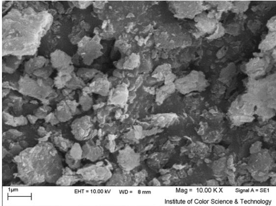
Figure 1a. SEM image of surface of the tonsil adsorbent (Scale: 1 micron).
