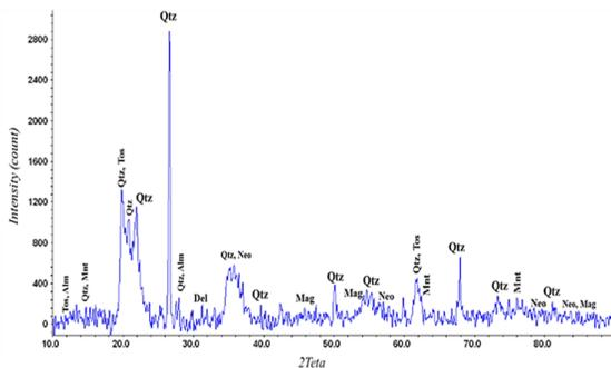
Figure 2. XRD graph of tonsil nano-particles.
