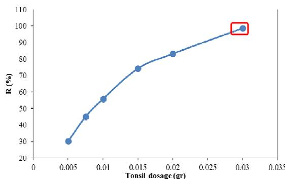
**Figure 5. Adsorption efficiency of tonsil at different concentrations, [dye] = 30 ppm.**
