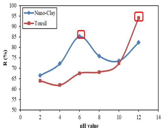
Figure 6. Effect of pH on CR18 adsorption onto tonsil and nano-clay.
