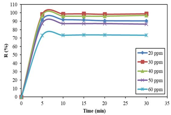
Figure 10. Effect of CR18 concentration on the adsorption efficiency of nano-clay.
