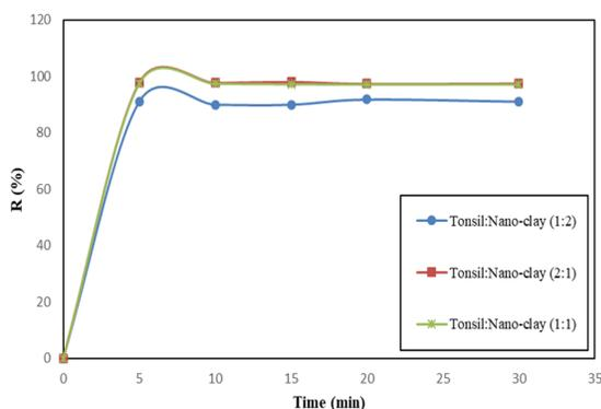
**Figure 22.** Effect of tonsil: nano-clay concentration ratios on the adsorption efficiency under optimum conditions of tonsil.
