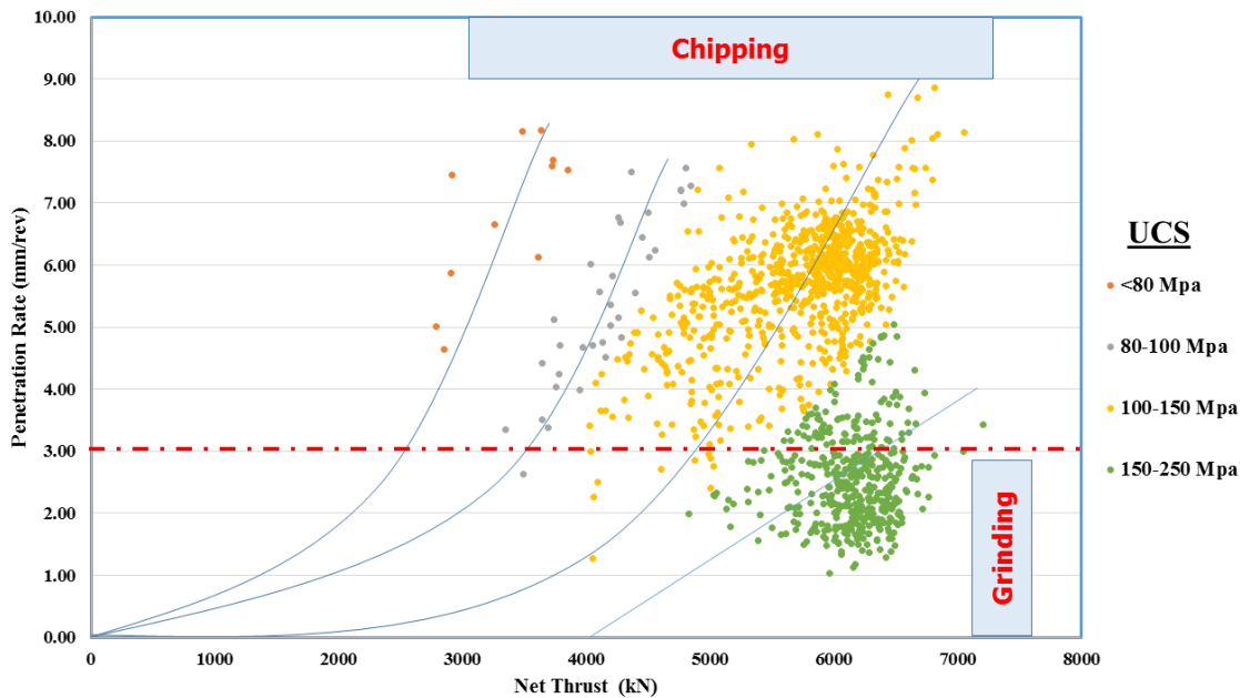
Figure 10. Relationships between net thrust force and penetration (P) for different UCS values.
