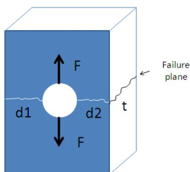
Figure 6. Parameters used for calculation of rock's direct tensile strength.
