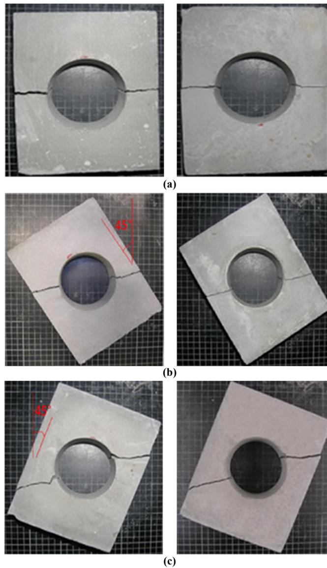
**Figure 5. Direct tensile failure pattern in specimens.**
