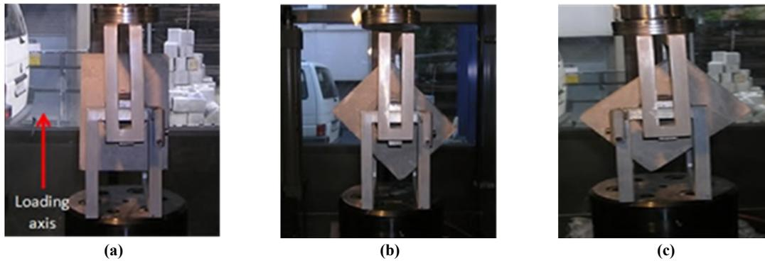
**Figure 4. Three loading configuration for the testing specimens: (a) located parallel to the loading axis, (b) turned  $45^\circ$  in a clockwise direction with respect to the loading axis, (c) turned  $45^\circ$  in counter-clockwise direction with respect to that of the load axis.**
