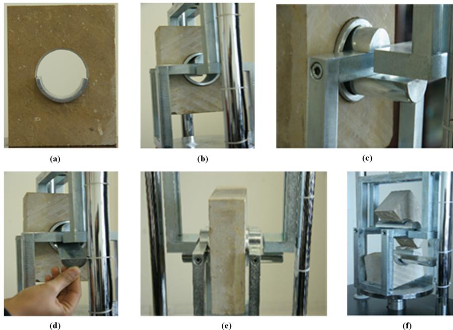
Figure 2. Setup procedure of CTLC device.
