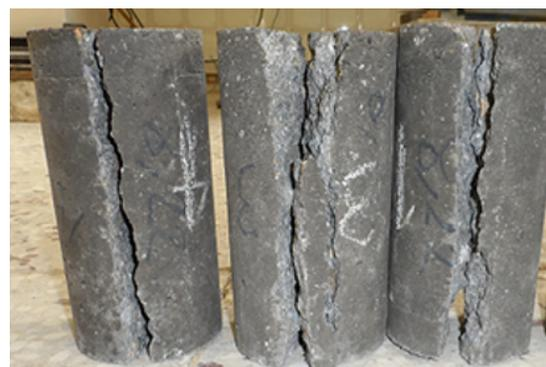
Figure 7. Failure pattern in experimental Brazilian tensile test.
