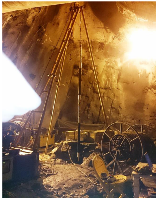
Figure 6. HF/HTPF test station at the top of the HF1 borehole.
