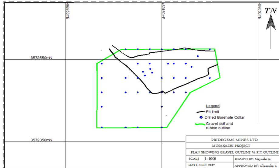
Figure 7. Plan showing rubble ore distribution.
