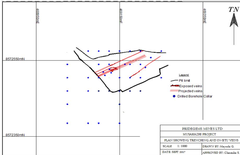
Figure 6. Plan showing projected in-situ quartz veins.
