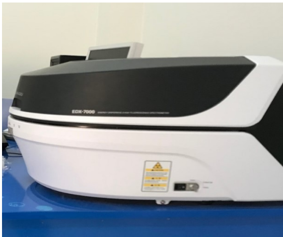
Figure 7. X-Ray Fluorescence spectrometer model EDX-7000.
