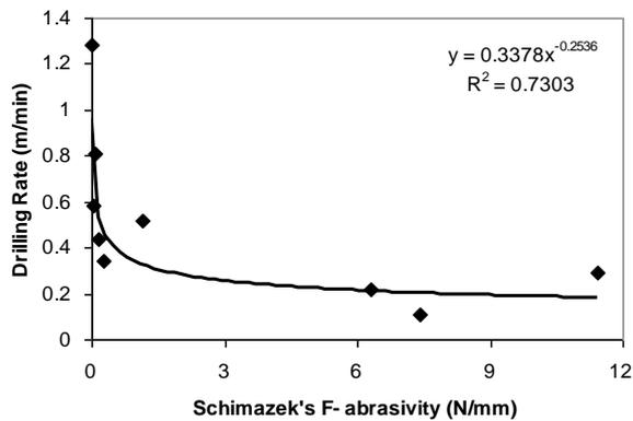
Figure 10. Drilling rate versus Schimazek's F-abrasivity
