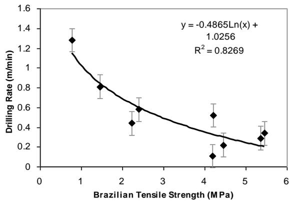
Figure 4. Drilling rate versus Brazilian tensile strength
