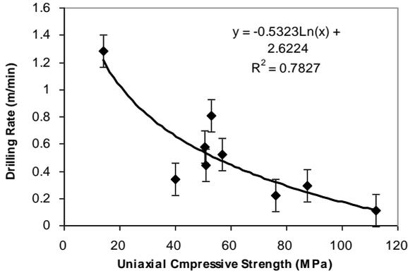
Figure 3. Drilling rate versus uniaxial compressive strength
