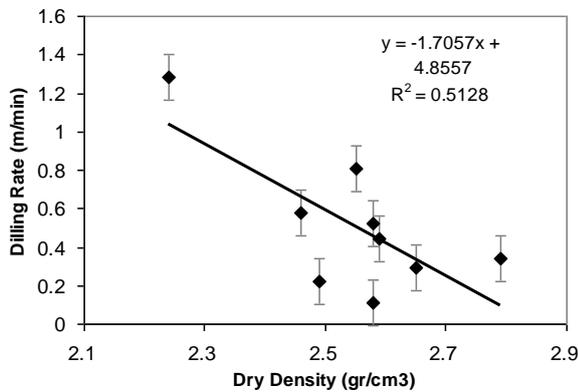
Figure 5. Drilling rate versus dry density
