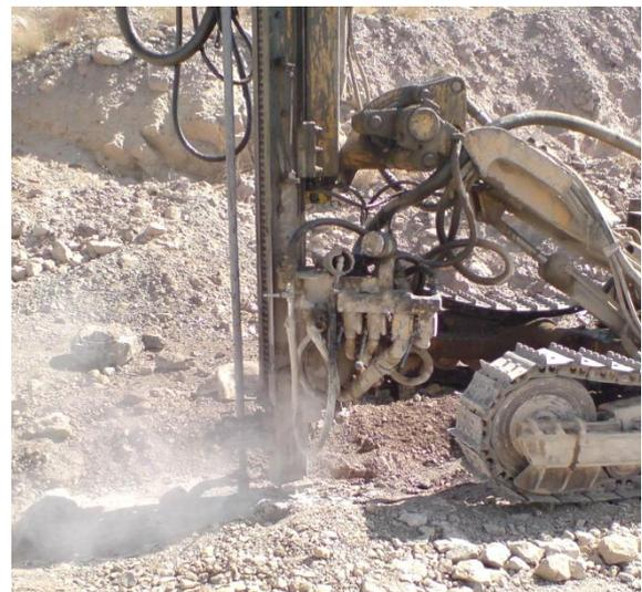
**Figure 2. Drilling machine while drilling the rock samples**
