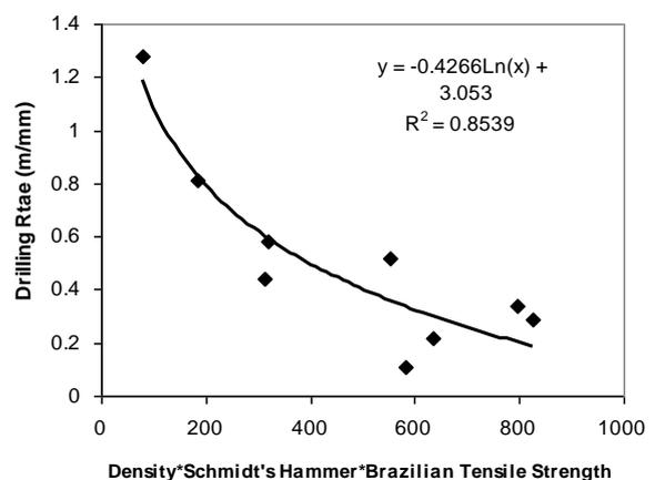
Figure 12. Drilling rate versus Density×Schmidt Hammer×Brazilian Tensile Strength
