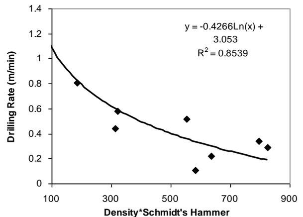
Figure 11. Drilling rate versus Density×Schmidt Hammer
