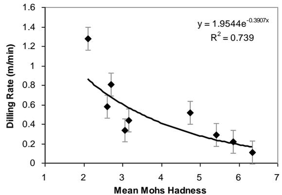
Figure 8. Drilling rate versus mean Mohs hardness
