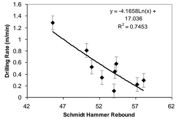
Figure 6. Drilling rate versus Schmidt hammer rebound
