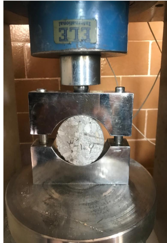
Figure 2. Brazilian test on the concrete specimens.
