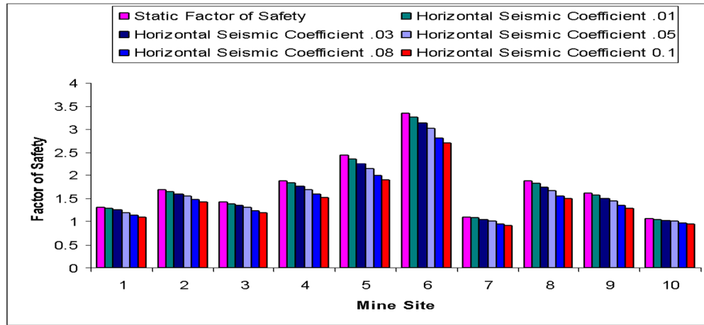
Figure 12. Increasing horizontal seismic coefficient showing decreasing factor of safety.
