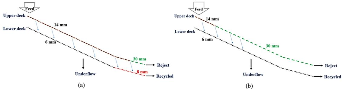
Figure 6. Wet double screen before (a) and after (b) modifications.
