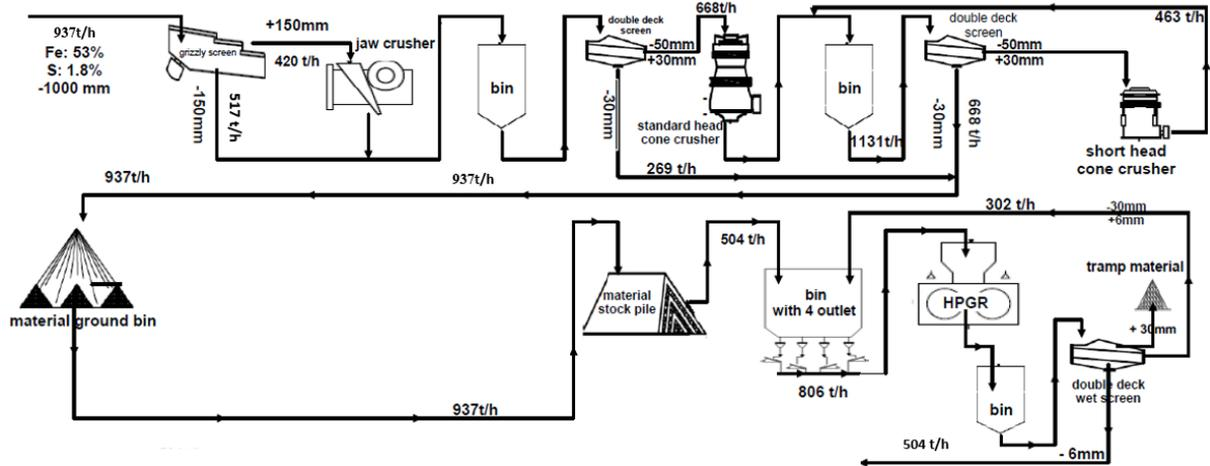
Figure 1. Iron ore crushing plant of Steel-Sirjan Iron Ore Complex.
