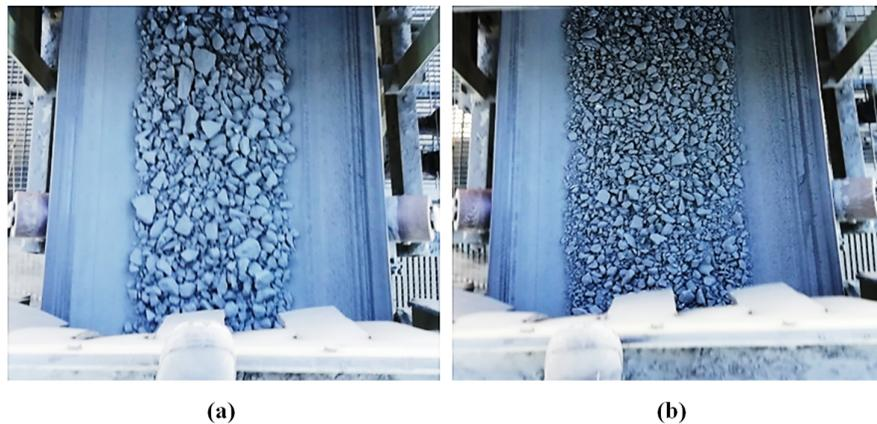
Figure 4. Product view of tertiary crusher in half-full (a) and choke fed operating (b) conditions.
