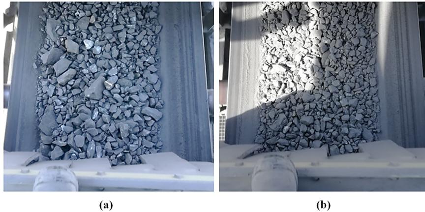
Figure 3. Product view of secondary crusher in half-full (a) and choke fed operating (b) conditions.
