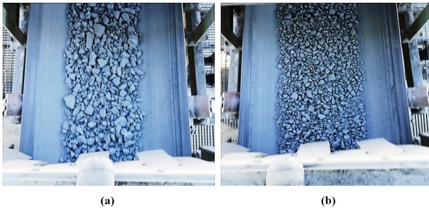
Figure 4. Product view of tertiary crusher in half-full (a) and choke fed operating (b) conditions.
