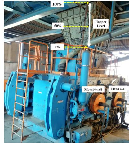
Figure 2. A view of HPGR and its hopper level.
