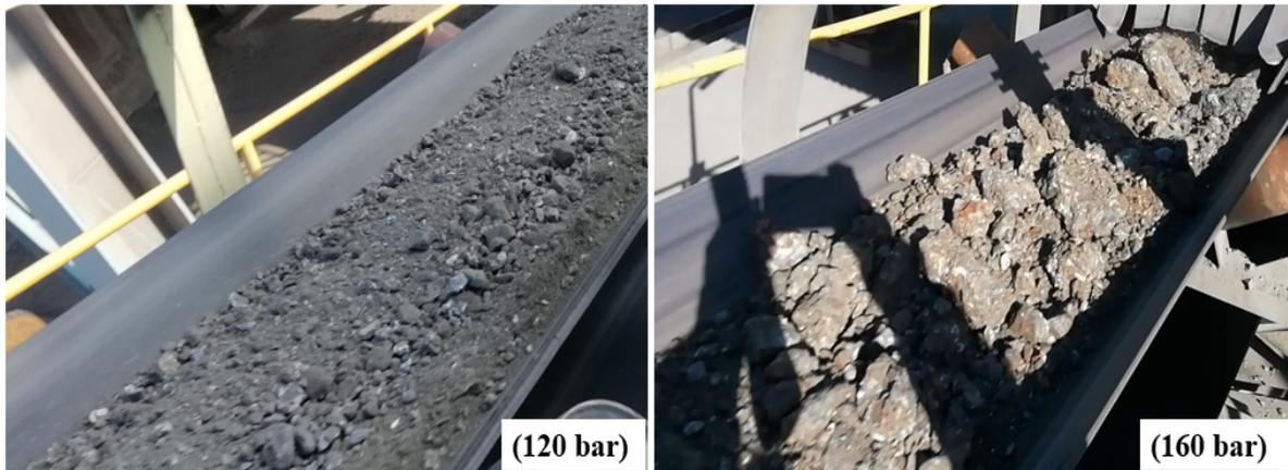
Figure 5. HPGR belt product in the operational pressures of 120 bar and 160 bar.
