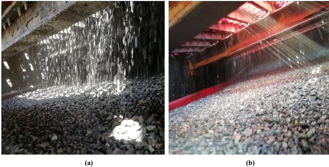
**Figure 8. Material spill on second deck before (a) and after (b) modifications.**
