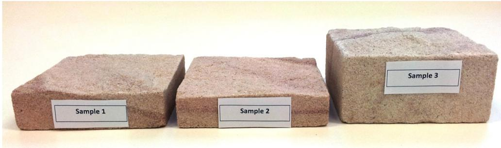
Figure 2. Three tensile joint surfaces of Hawkesbury sandstone having different joint roughness coefficient ( $JRC$ ) values ( $JRC_{Sample\ No.\ 1} = 13.2$ ,  $JRC_{Sample\ No.\ 2} = 12.5$ , and  $JRC_{Sample\ No.\ 3} = 17.3$ ).
