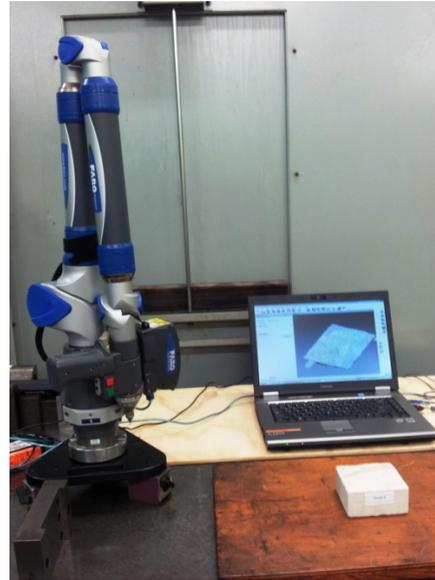
Figure 3. Digitising a typical joint surface using FARO Laser ScanArm.
