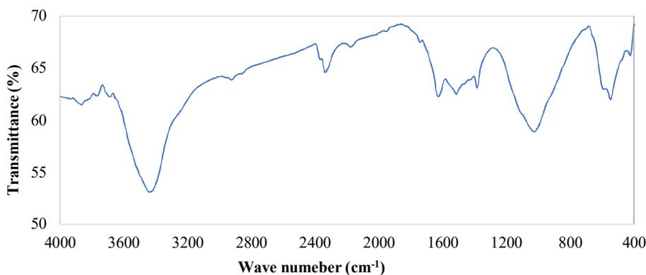
Figure 4. FT-IR spectrum of biosynthesized CdO NPs using *Ferula*.
