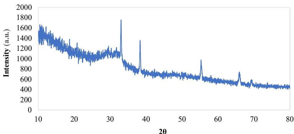
Figure 3. XRD pattern of synthesized CdO NPs using *Ferula*.
