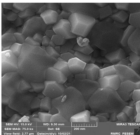
Figure 5. FE-SEM micrograph of synthesized CdO NPs using *Ferula*.
