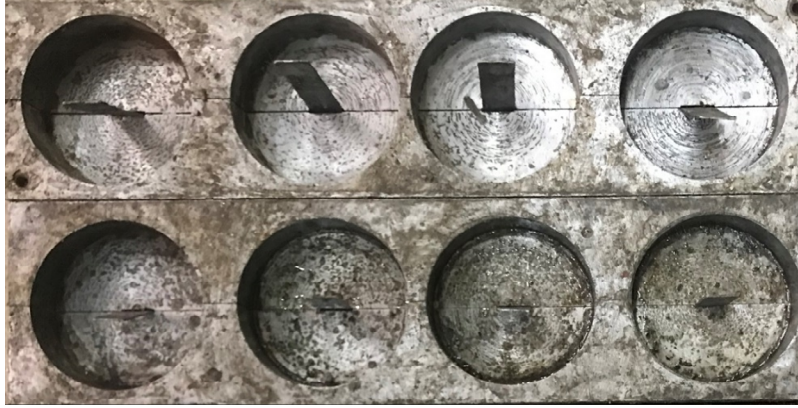
Figure 3. Molds constructed to prepare SNBD concrete specimens.
