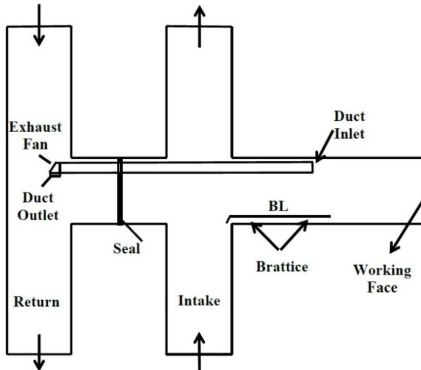
Figure 2. Computational model in top view.
