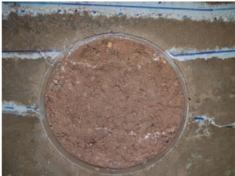
Figure 11. Drilling hole in front wall of physical model and soil before drilling.
