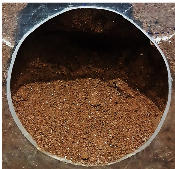
Figure 30. Collapse and blocking of tunnel.
