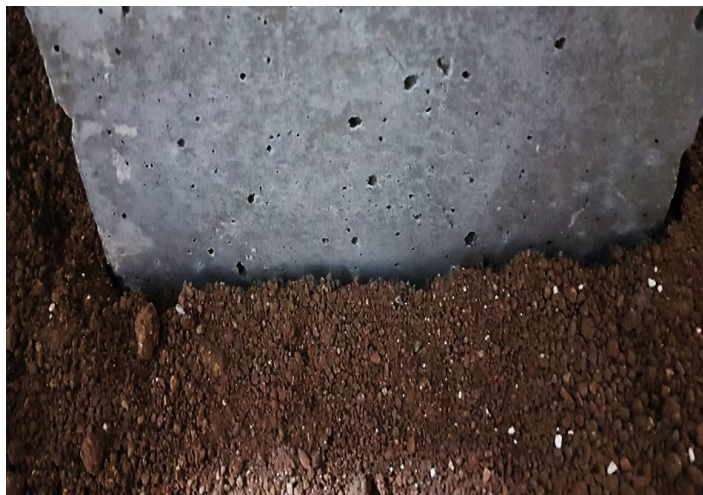
Figure 20. Blocks sinking into soil.
