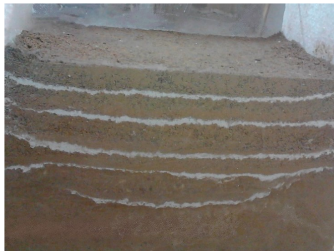
Figure 9. Five white layers created in physical tank (back-view).
