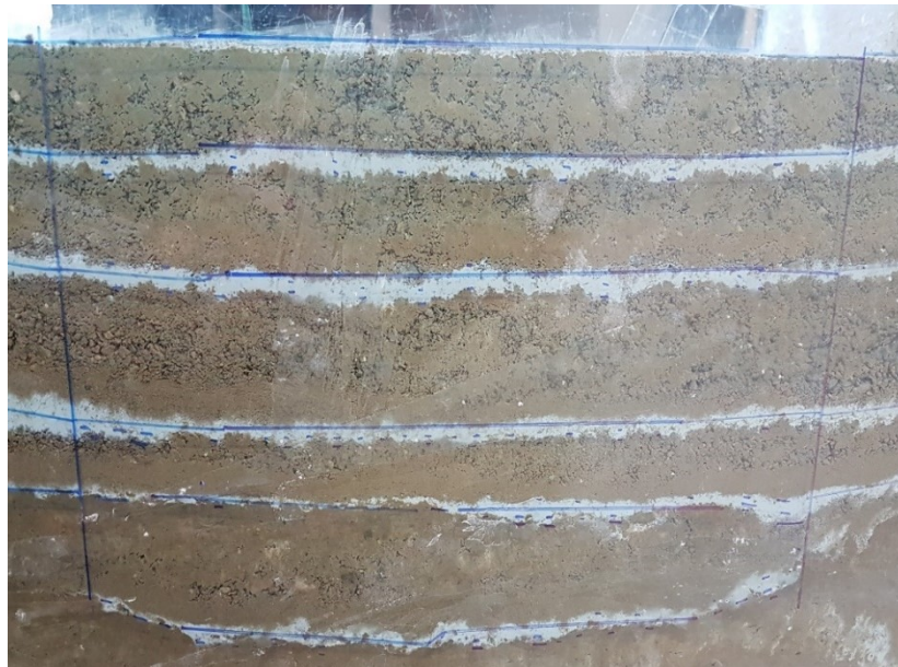
Figure 10. Six blue indicator lines on wall of physical model (rear- view).
