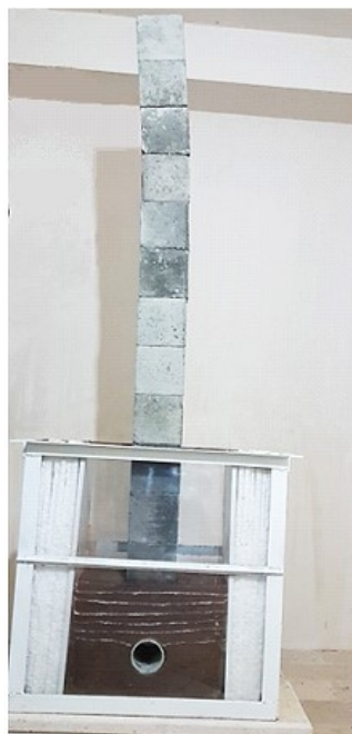
Figure 23. Applying twelfth concrete block to tunnel with segmental maintenance.
