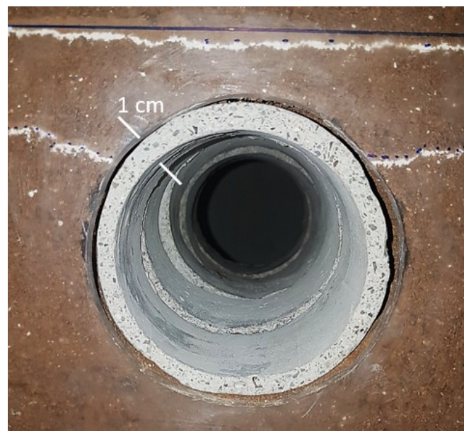
Figure 19. Maintenance and stabilization of collapsing tunnel with segmentation method.
