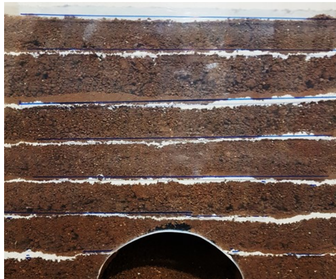
Figure 18. Displacement of white layers relative to blue index lines after settlement (white layers came under index lines).
