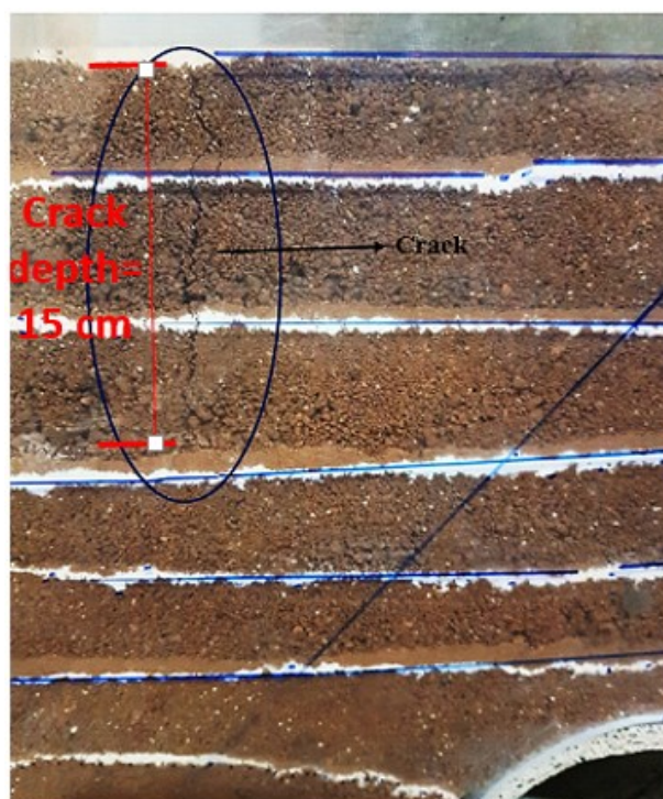
Figure 27. Deepest vertical crack.
