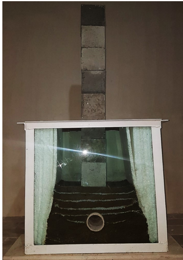
Figure 14. Loading equivalent to 64 kg on tunnel maintained with segments.
