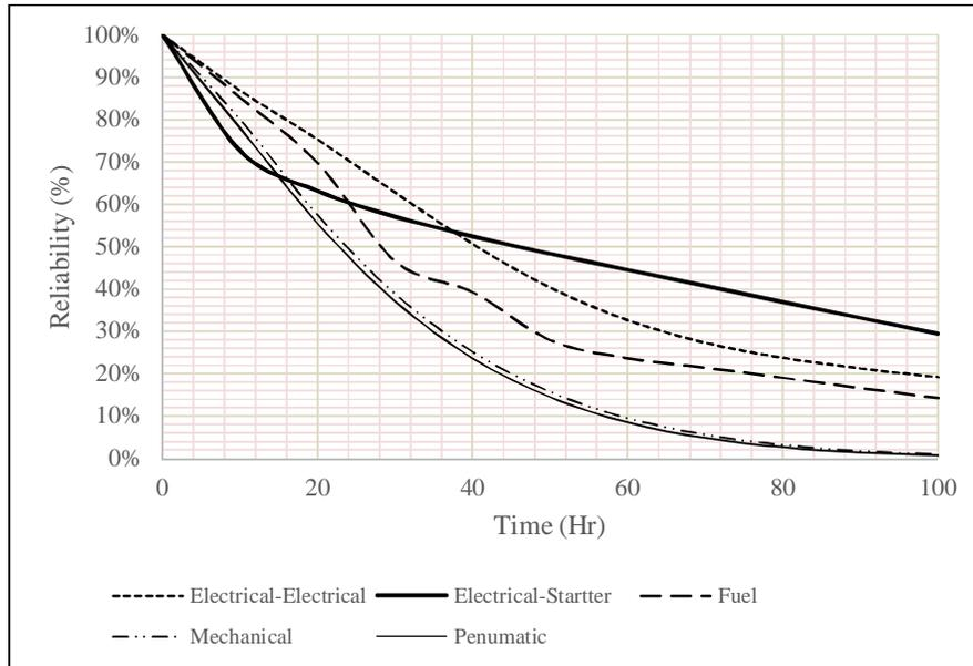
Figure 6. Reliability of various modes of system failure.
