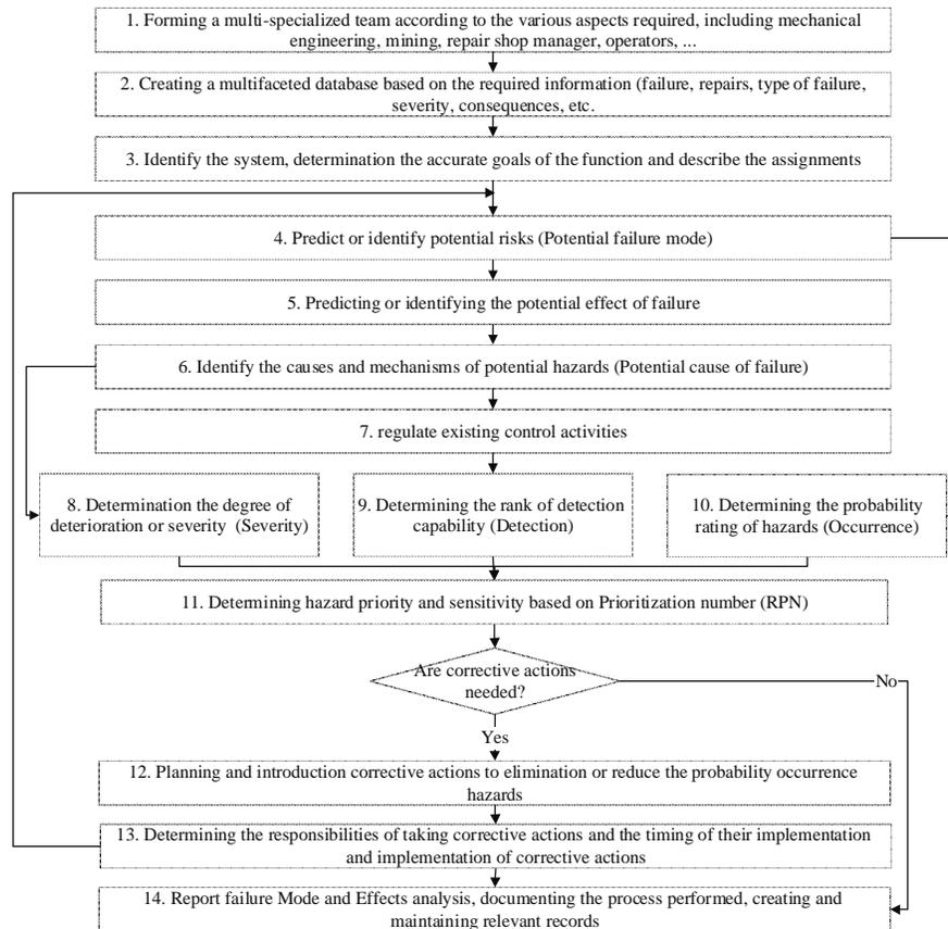
Figure 2. Implementation algorithm of Failure Mode and Effects Analysis [65], [66].
