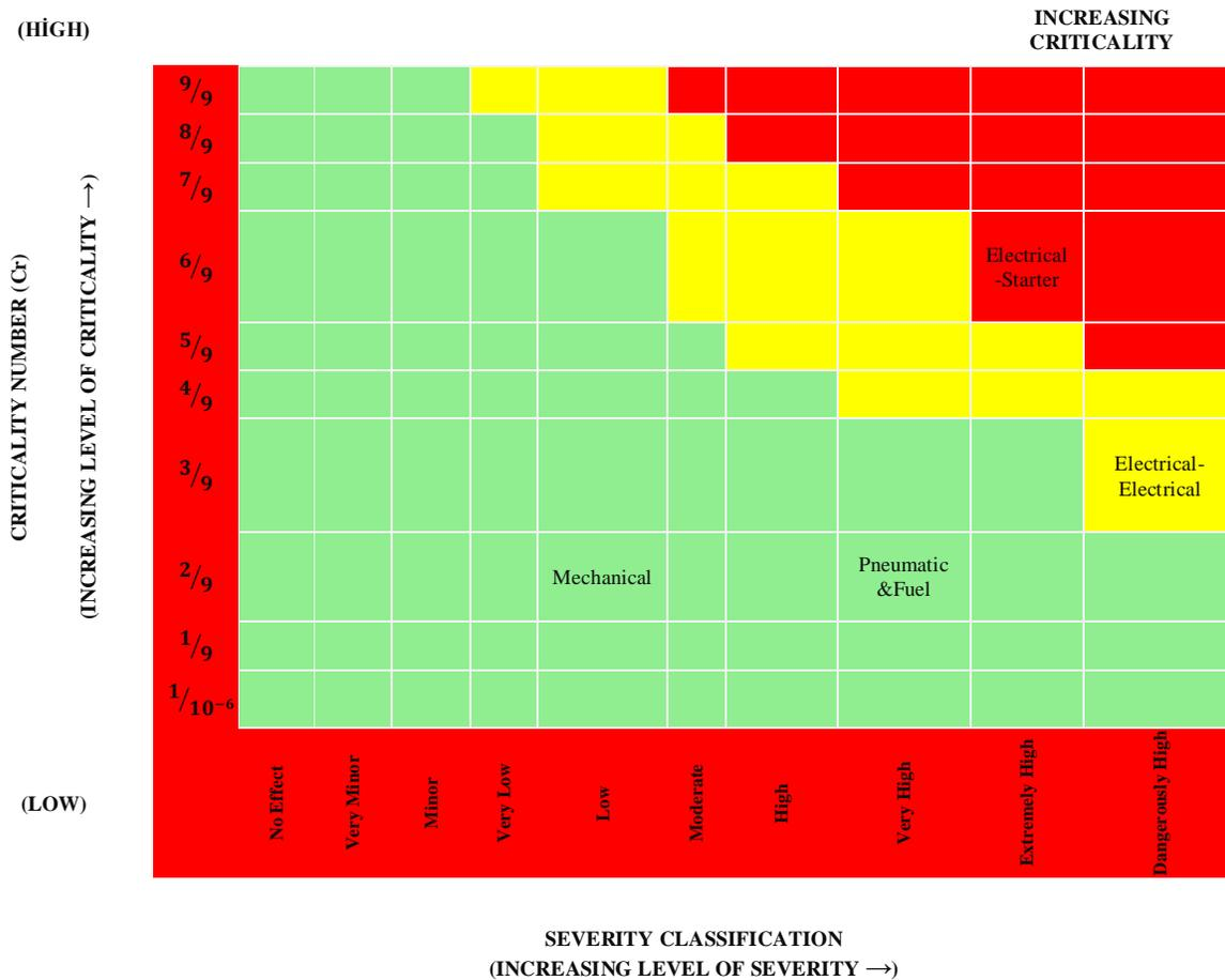
Figure 10. Qualitative criticality matrix for different failure modes (intensity-criticality).
