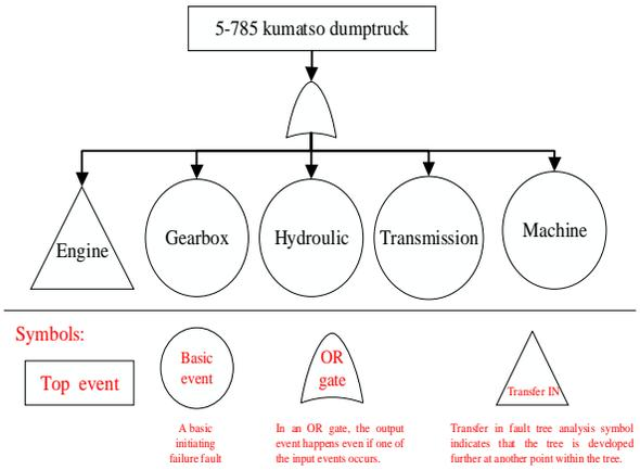
Figure 3. 5-785 Komatsu dump truck FTA chart.
