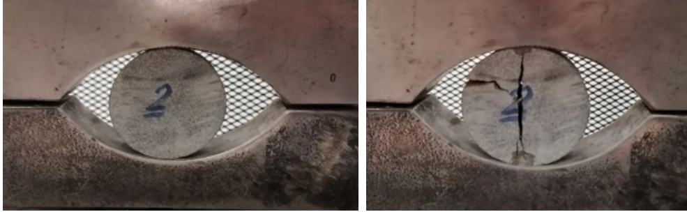
Figure 6. Fine-grained sandstone samples under the Brazilian test.
