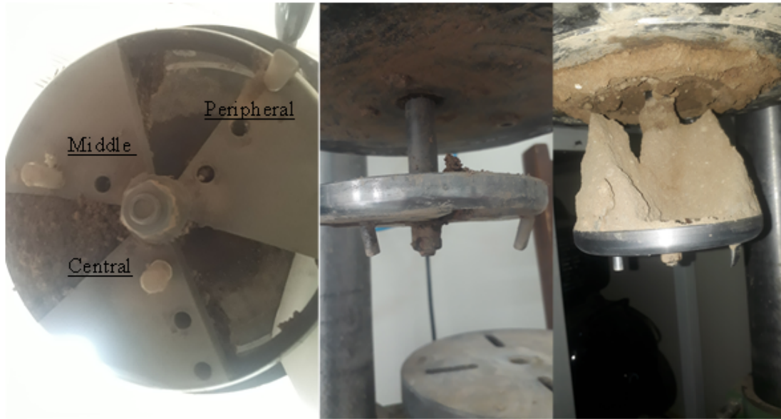
Figure 8. Position of cutting tools on the cutterhead.
