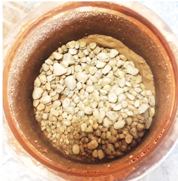
Figure 20. Soil chamber in the LCPC test after the end of testing on the standard soil sample.
