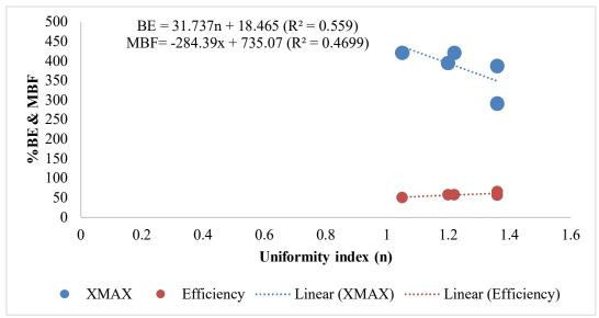
Figure 5. Relationship between MBF, BE, and uniformity index.
