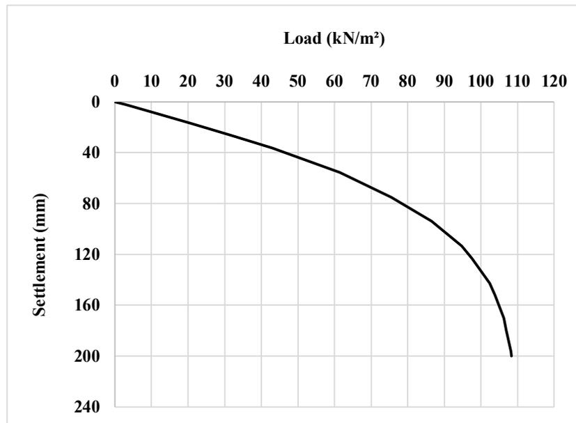
Figure 4. Load-displacement curve of unreinforced soil under the raft foundation.
