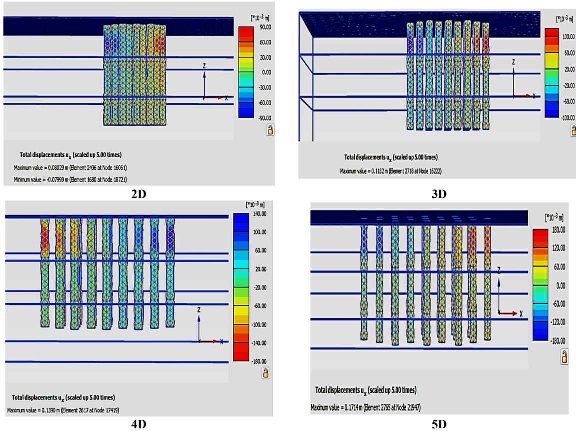
Figure 7. Displacement contours of stone columns in triangular arrangement with spacing ranging from 2D to 5D.
