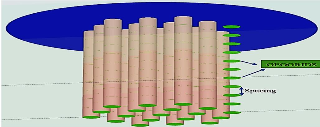
Figure 12. Circular geogrids along the length of stone columns.
