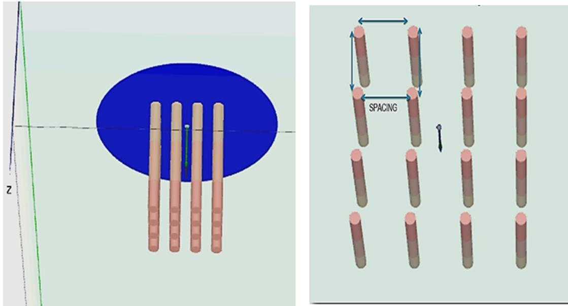
Figure 8. Stone columns arranged in a square pattern.
