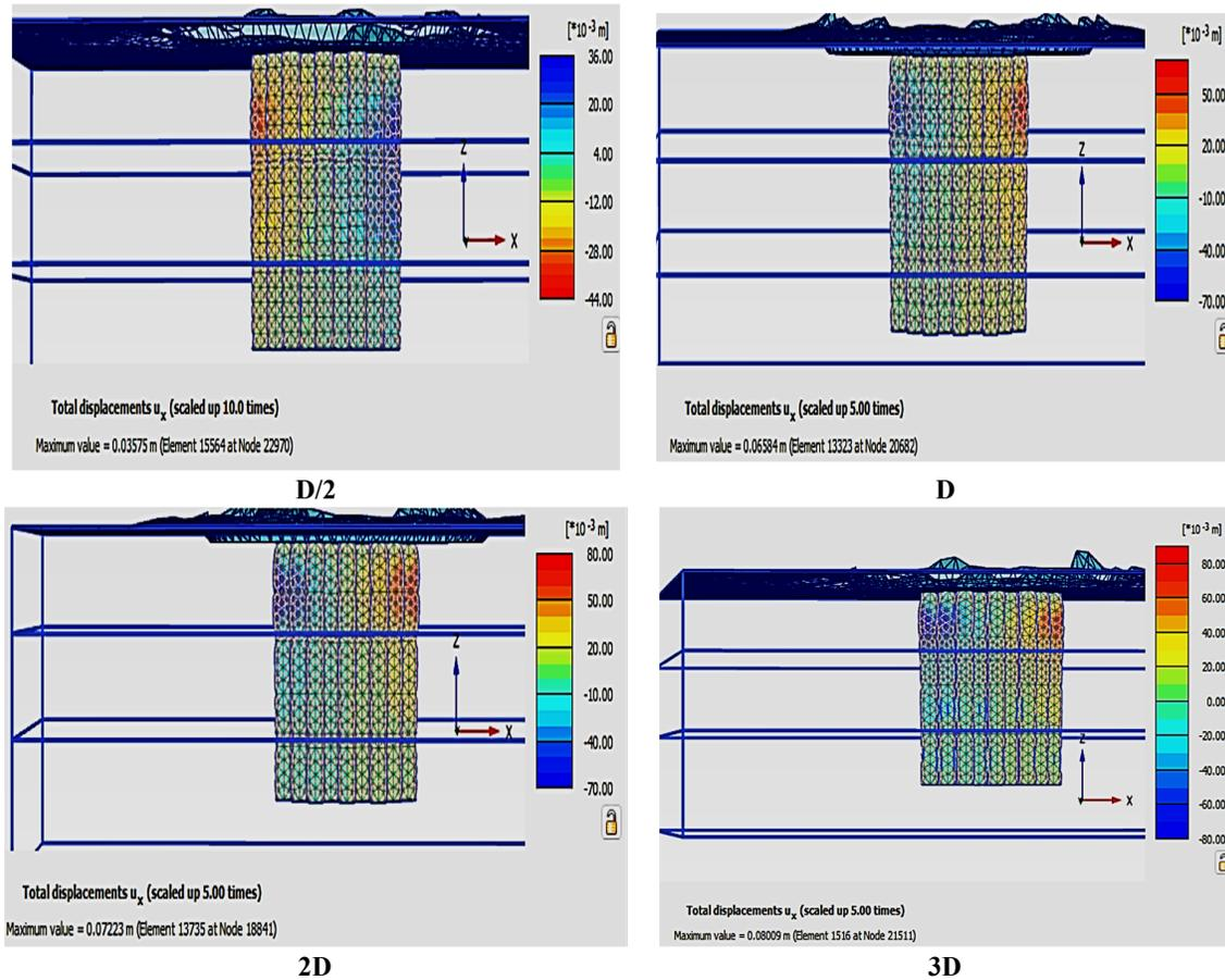
Figure 14. Displacement contours of HRSCs with geogrid spacing ranging from D/2 to 3D.
