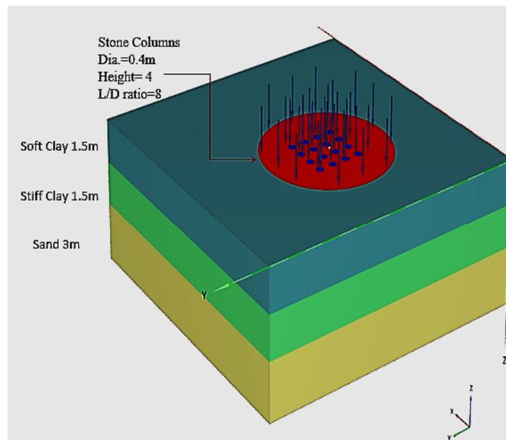
Figure 1a. Symmetrical square arrangement of stone columns.
