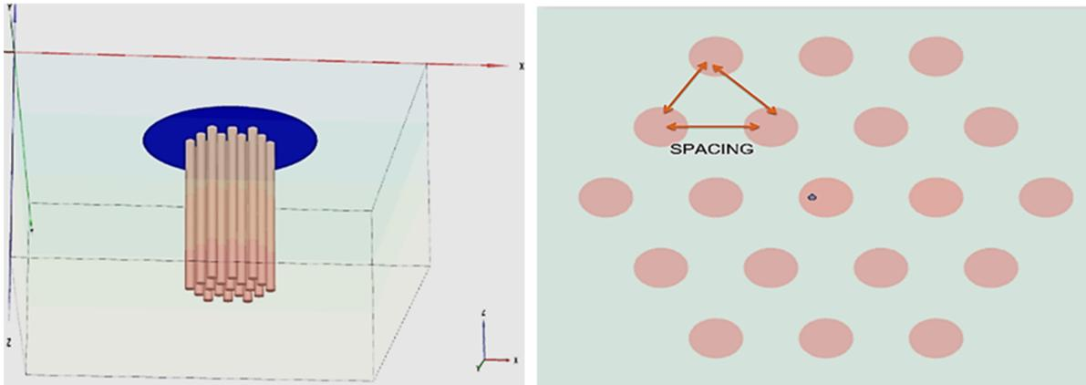
Figure 5. Stone columns arranged triangularly.
