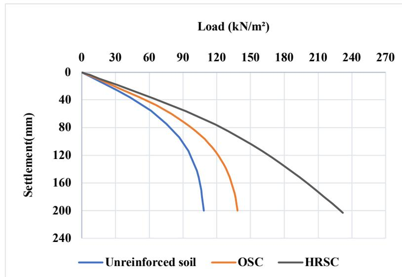
Figure 15. Comparative load settlement curve.
