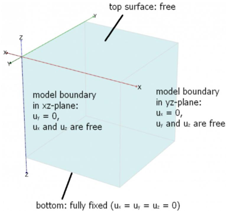
**Figure 1b. Boundary conditions of the model.**
