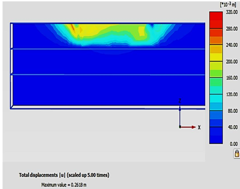
Figure 3. Overall footing displacement contour of the raft on the stratified soil.
