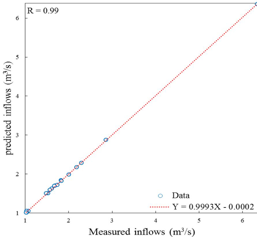
Figure 4. The linear regression plot of the field measured inflow versus the predicted inflow for the testing stage including R value by ANN-GA.
