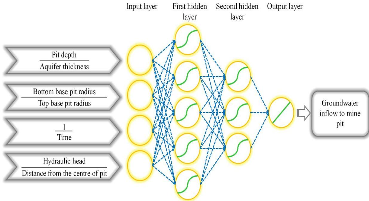
Figure 2. ANN-GA architecture with 4-5-3-1 arrangement comprising hyperbolic tangent and linear transfer functions.
