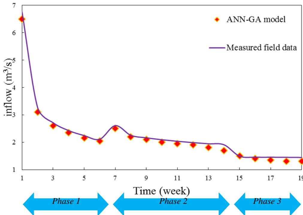
Figure 5. Comparison of filed data with ANN-GA model results for groundwater inflow to Kolahdarvazeh mine pit during its advance.
