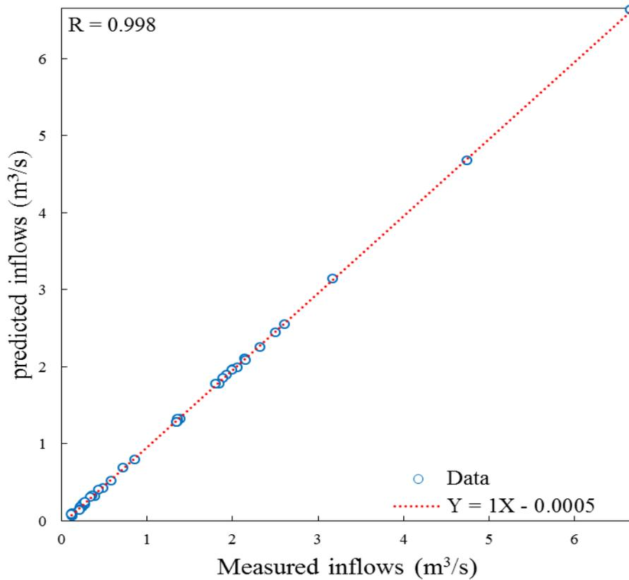
Figure 3. The linear regression plot of the field measured inflow versus the predicted inflow for the training stage including R value by ANN-GA.
